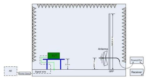
Radiated tests above 1GHz
