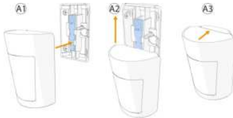
Figure 11: Attaching the device to the corner bracket
