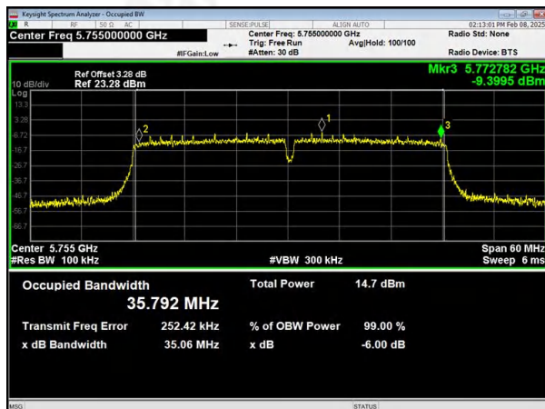
(802.11n40) PSD plot on channel 151
