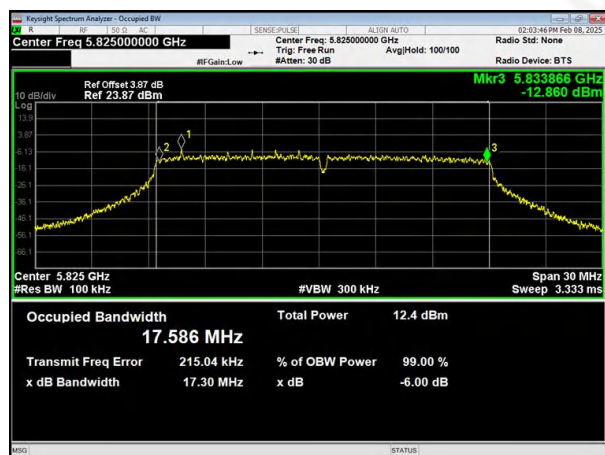
(802.11n20) 6dB Bandwidth plot on channel 165
