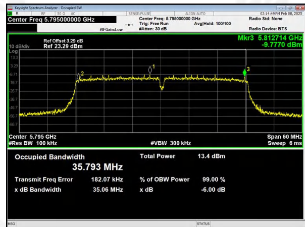
(802.11ac40) PSD plot on channel 159
