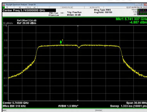
(802.11ac20) PSD plot on channel 157
