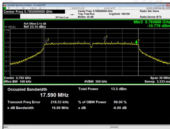
(802.11ac20) 6dB Bandwidth plot on channel 165
