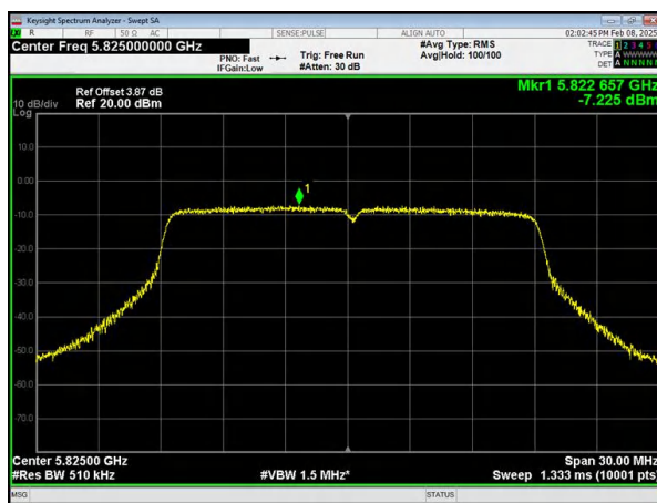
(802.11ac20) PSD plot on channel 165
