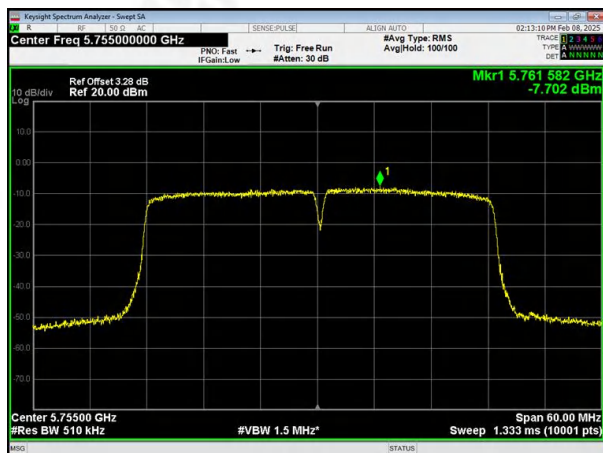
(802.11n40) PSD plot on channel 159
