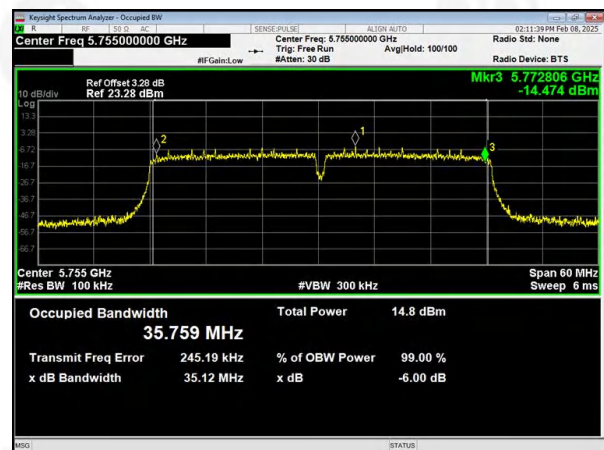
(802.11ac40) PSD plot on channel 151
