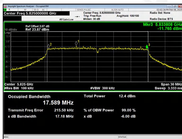
(802.11ac20) 6dB Bandwidth plot on channel 165
