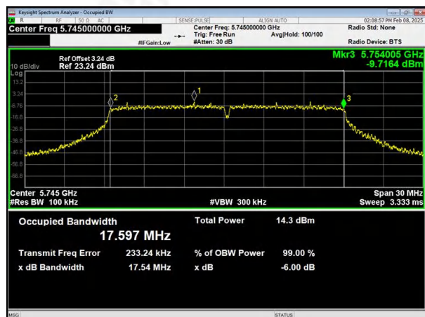
(802.11n20) 6dB Bandwidth plot on channel 149
