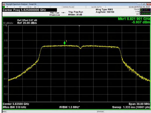
(802.11a) PSD plot on channel 165
