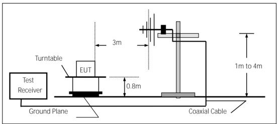
(c) For radiated emissions above 1000MHz
