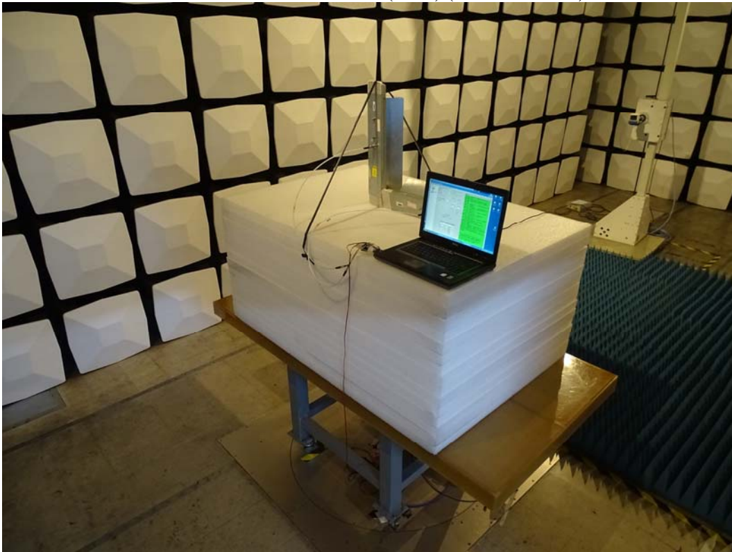
Front View of Radiated Test (Horn) (Sector Antenna)
