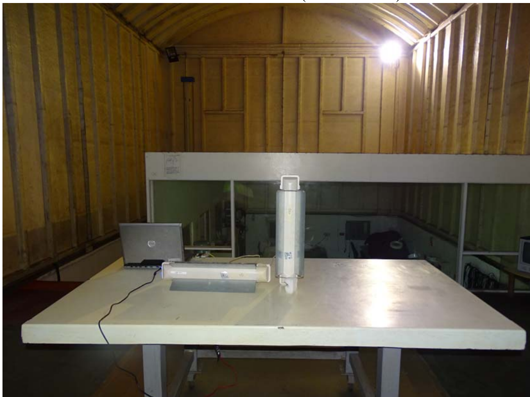
Back View of Radiated Test (Sector Antenna)
