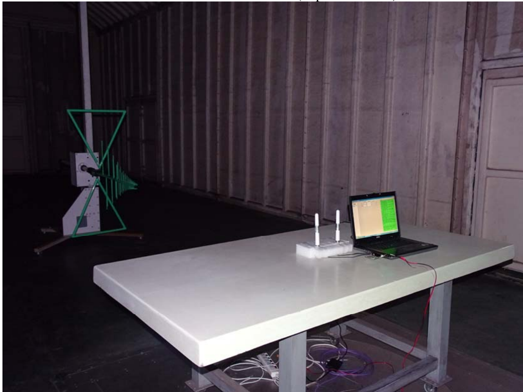
Front View of Radiated Test (Dipole Antenna)
