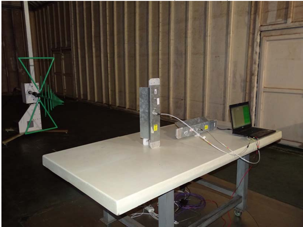
Front View of Radiated Test (Sector Antenna)
