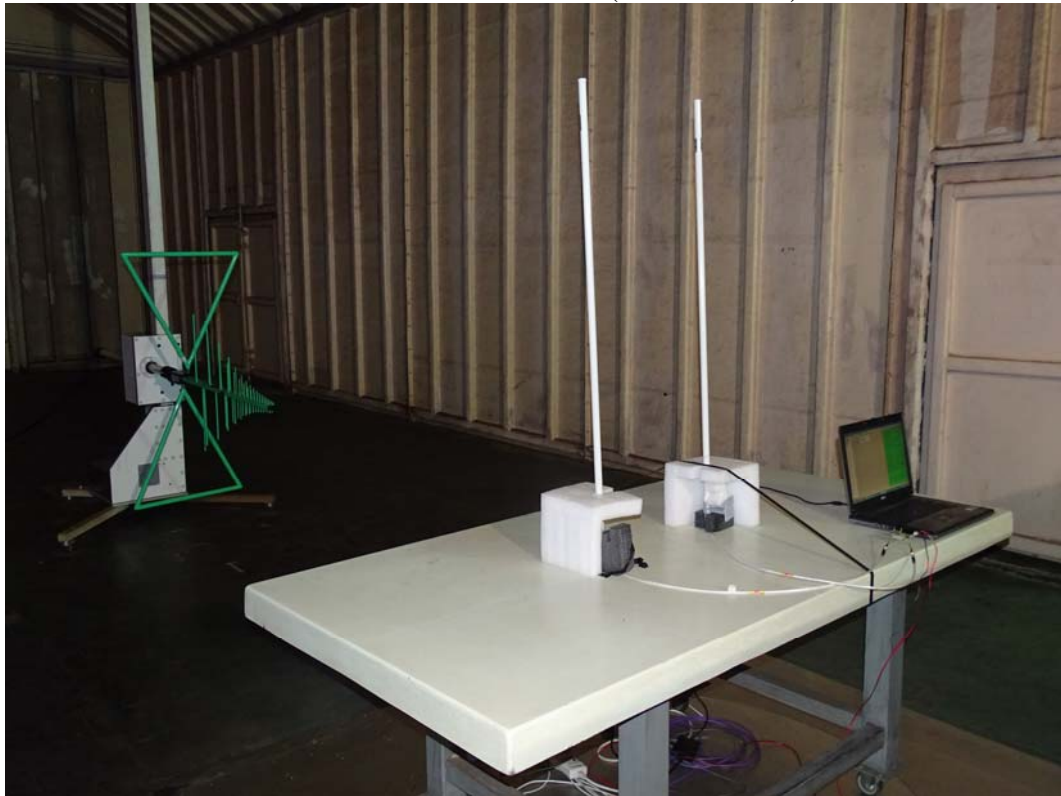
Front View of Radiated Test (Omni Antenna)
