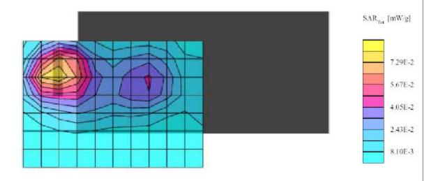
Verifone, Omni 56XXG (GPRS 1900, Top Side of the DUT faced toward and 1.5 cm separation to flat phantom, Ambient Temp = 23 Deg C, Liquid Temp = 22 Deg C, 8/12/04) SAM Phantom; Flat Section; Position: (90°,90°); Frequency: 1900 MHz
