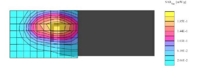
Verifone, Omni 56XXG (GPRS 850, Back Side of the DUT faced toward and 1.5 cm separation to flat phantom, Ambient Temp = 23 Deg C, Liquid Temp = 22 Deg C, 8/12/04) SAM Phantom; Flat Section; Position: (90°,90°); Frequency: 836 MHz
