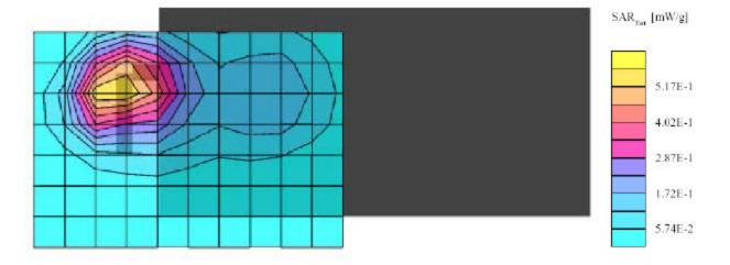
Verifone, Omni 56XXG (PCS 1900, Top Side of the DUT faced toward and 1.5 cm separation to flat phantom, Ambient Temp = 23 Deg C, Liquid Temp = 22 Deg C, 8/12/04)
