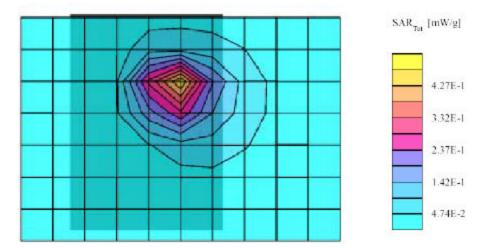
Verifone, Omni 56XXG (GPRS 1900, Back Side of the DUT faced toward and 1.5 cm separation to flat phantom, Ambient Temp = 23 Deg C, Liquid Temp = 22 Deg C, 8/12/04)
