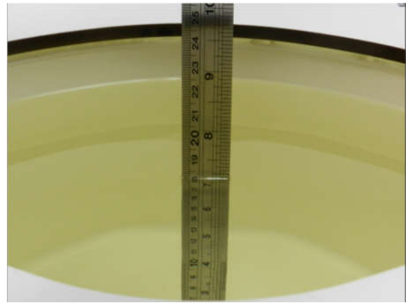
Fig 11.2 Photo of Liquid Height for Body SAR
