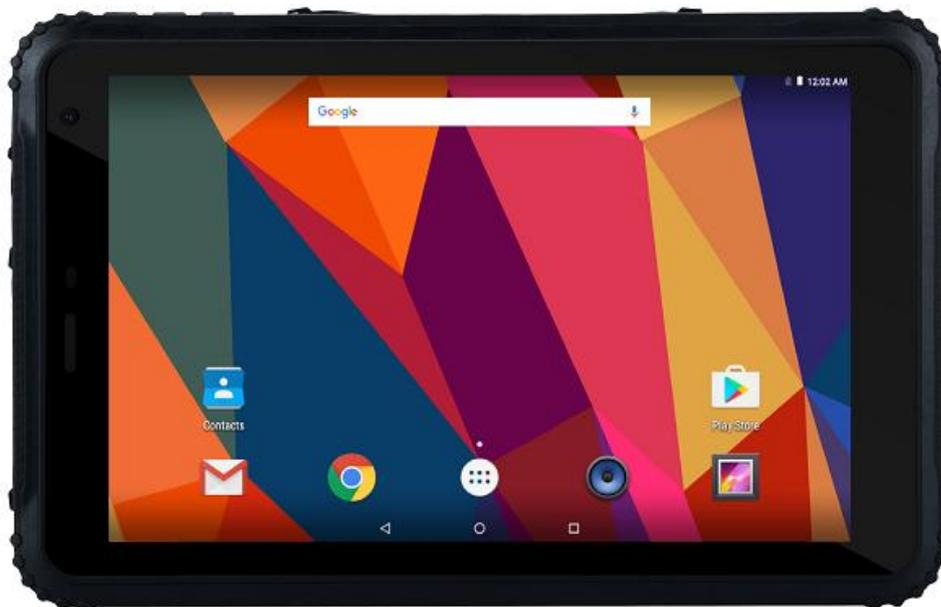
**10.Front camera/light sense:** camera can take picture, video.light sense can adjust Luminance automatically.
