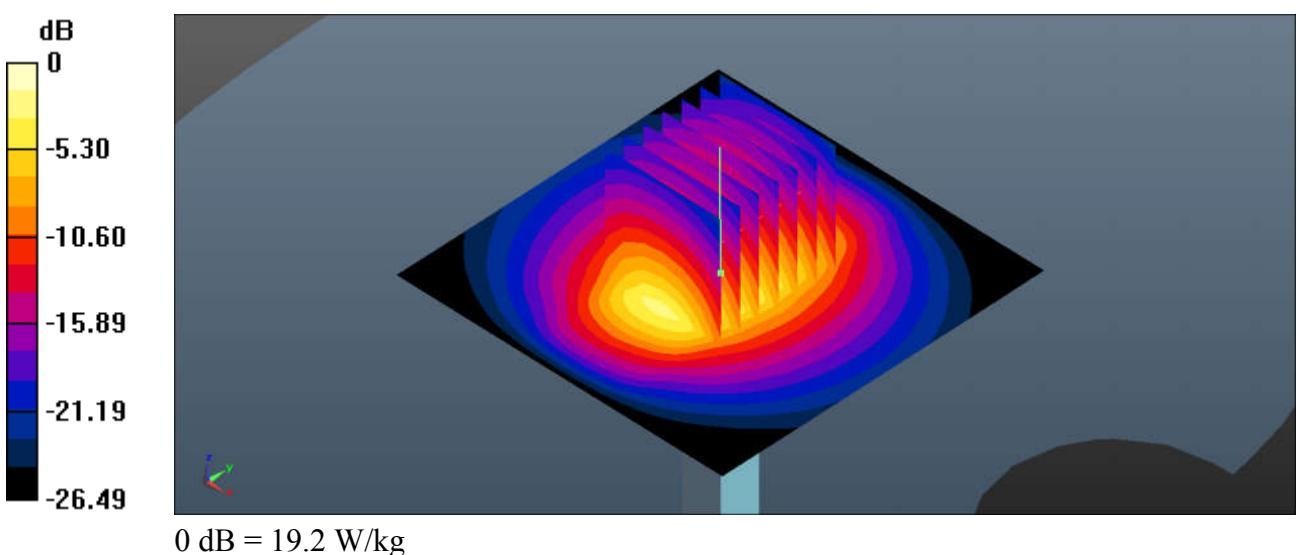
**System Check\_Body\_2600MHz****DUT: D2600V2 - SN:1061**
