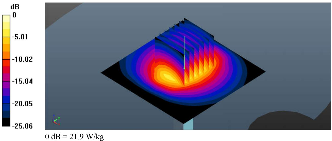
**System Check\_Head\_5250MHz****DUT: D5GHzV2-SN:1006**
