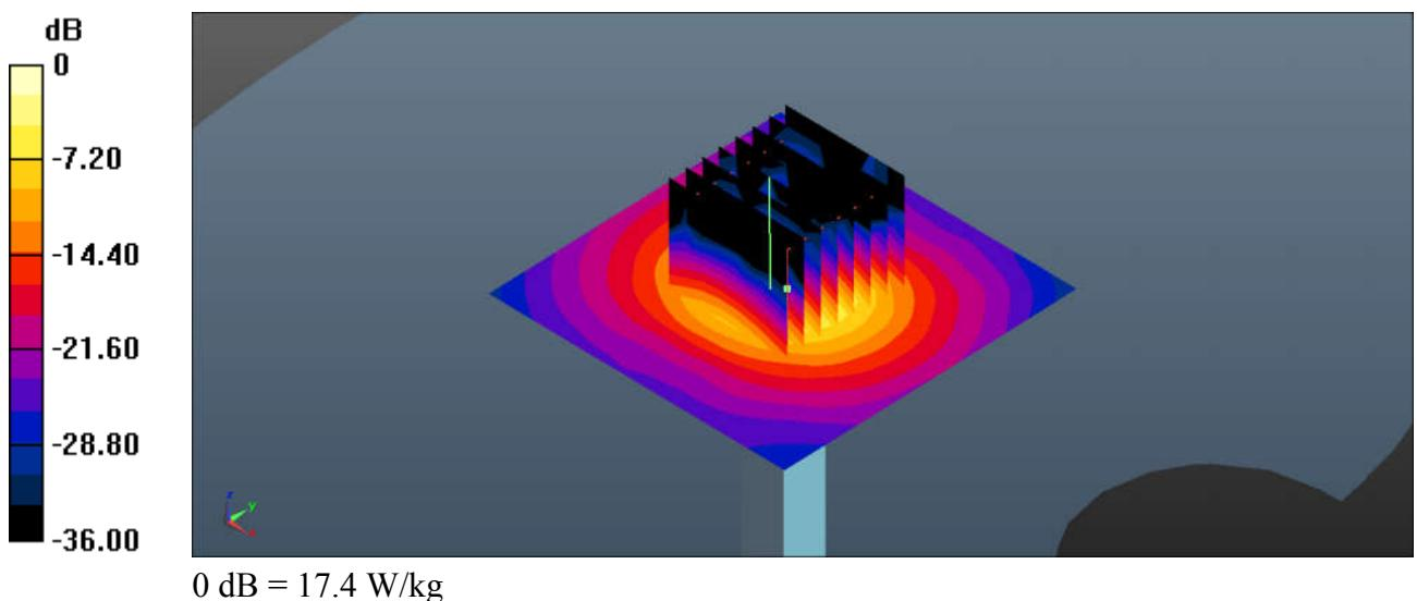
**System Check\_Body\_5600MHz****DUT: D5GHzV2-SN:1006**
