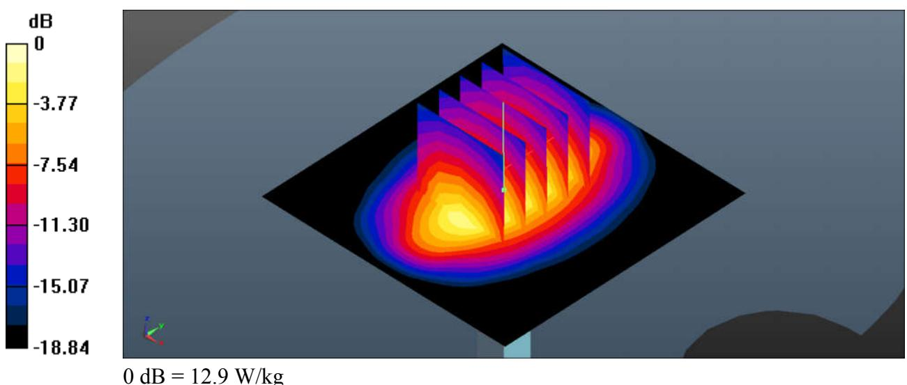
**System Check\_Body\_1900MHz****DUT: D1900V2 - SN:5d170**
