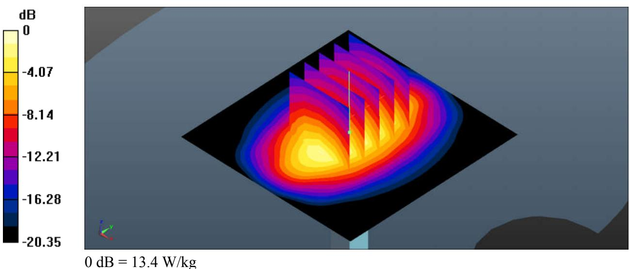
**System Check\_Head\_1900MHz****DUT: D1900V2 - SN:5d170**
