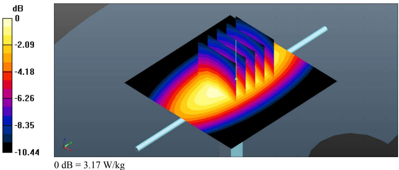
**System Check\_Body\_1750MHz****DUT: D1750V2 - SN:1090**
