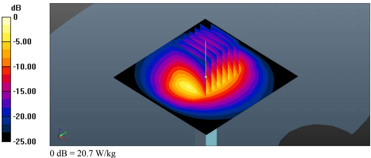
**System Check\_Head\_2600MHz****DUT: D2600V2 - SN:1061**
