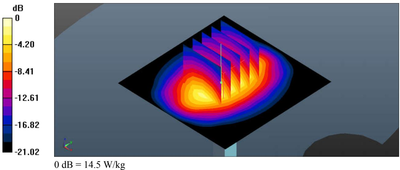
**System Check\_Head\_2450MHz****DUT: D2450V2 - SN:908**
