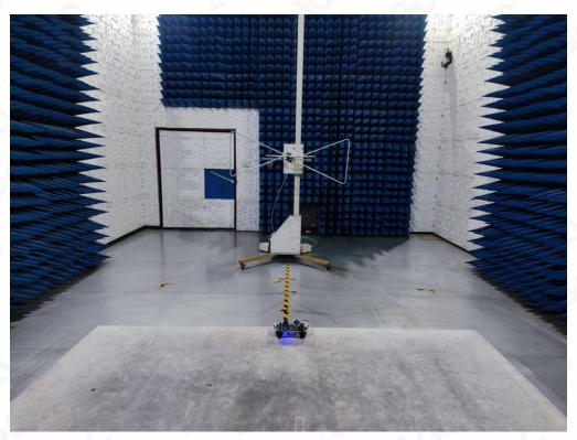
RADIATED EMISSION TEST SETUP ABOVE 1GHz
