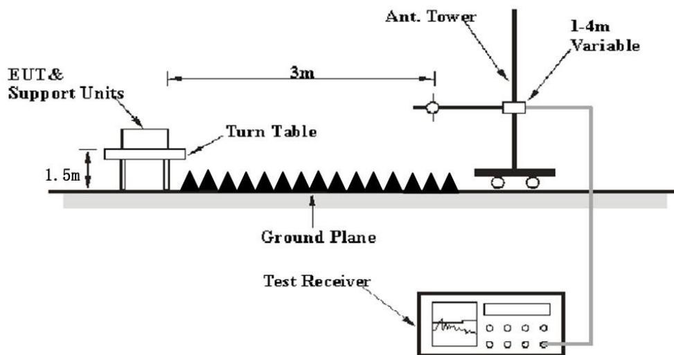
The radiated emission and out of band emission tests were performed in the 3 meters chamber test site, using the setup accordance with the ANSI C63.10-2013. The specification used was the FCC 15.209/15.205 and FCC 15.249 limits.
