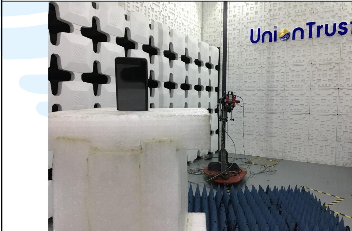
Radiated emission Test Setup (Above 1 GHz)
