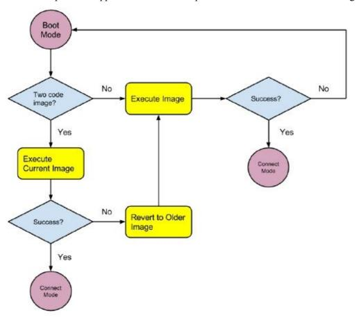
The MWA1221 would be in Boot Mode when power is first applied or a reboot/restart of code image has occurred.
