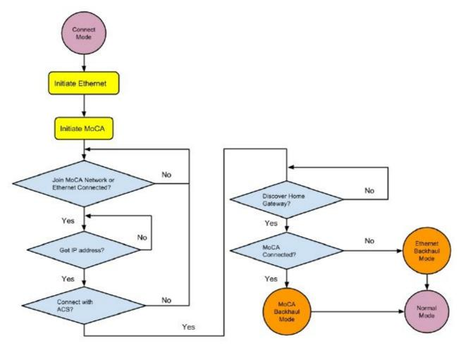
MWA1221 would transition to MoCA Backhaul Mode or Ethernet Backhaul Mode if the product has successfully entered Connect Mode.
