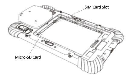
Please insert the SIM card and the MicroSD card in the direction of the diagram.
