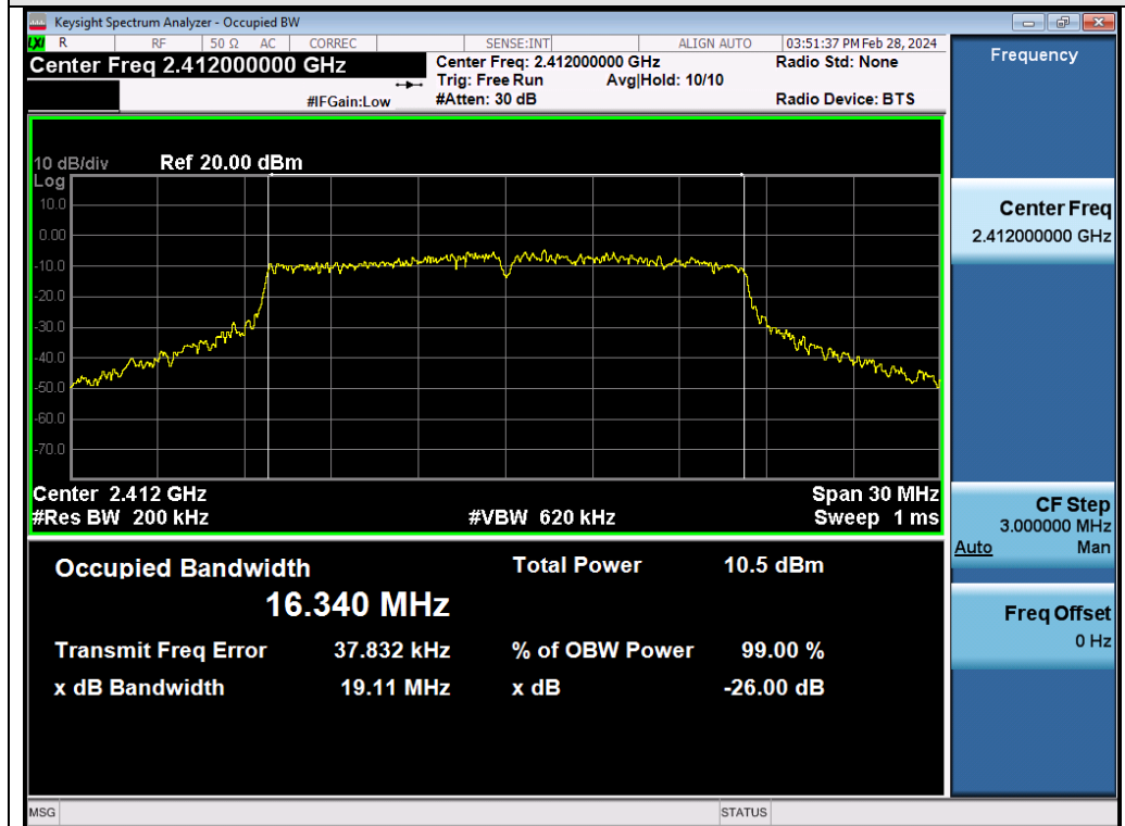
Test_Graph_802.11g_ANT1_2412_6Mbps_OBW
