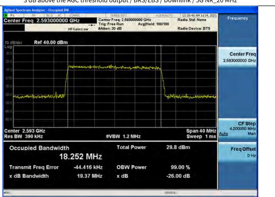
3 dB above the AGC threshold output / BRS/EBS / Downlink / 5G NR\_20 MHz
