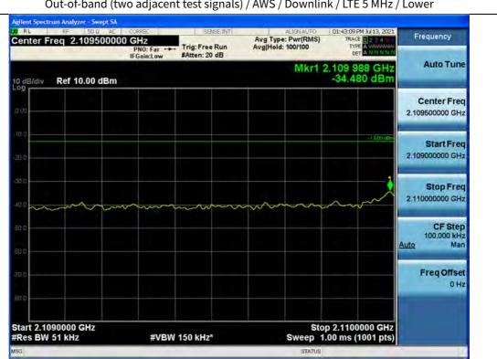
Out-of-band (two adjacent test signals) / AWS / Downlink / LTE 5 MHz / Lower
