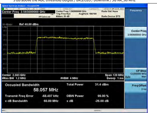
3 dB above the AGC threshold output / BRS/EBS / Downlink / 5G NR\_60 MHz
