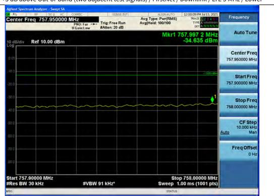
+3 dB above Out-of-band (two adjacent test signals) / FirstNet / Downlink / LTE 5 MHz / Lower
