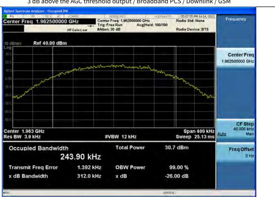
3 dB above the AGC threshold output / Broadband PCS / Downlink / GSM
