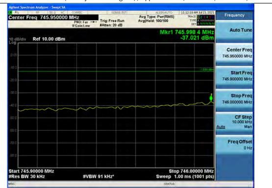
+3 dB above Out-of-band (two adjacent test signals) / Upper 700 MHz / Downlink / LTE 5 MHz / Lower
