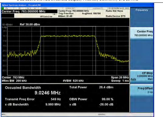
3 dB above the AGC threshold output / FirstNet / Downlink / LTE 10 MHz
