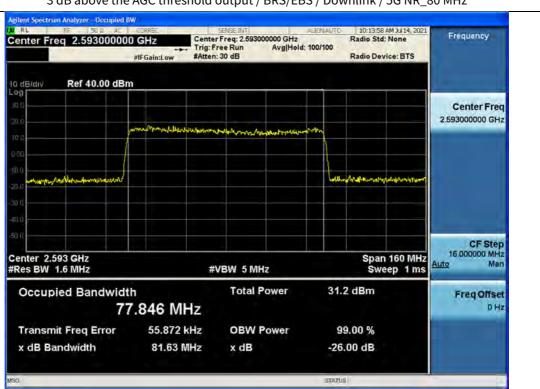
3 dB above the AGC threshold output / BRS/EBS / Downlink / 5G NR\_80 MHz
