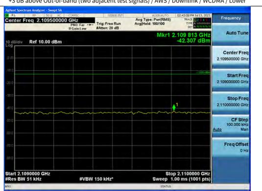
+3 dB above Out-of-band (two adjacent test signals) / AWS / Downlink / WCDMA / Lower
