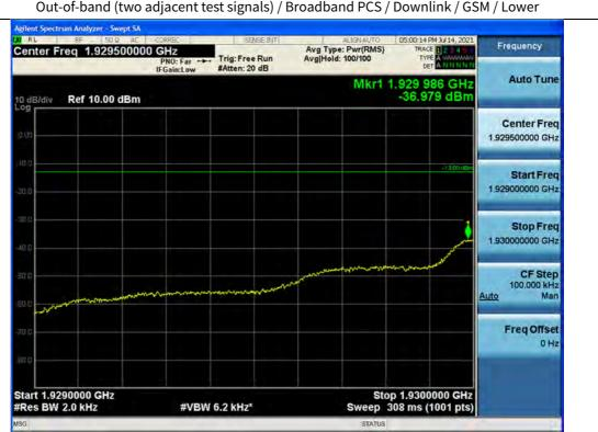
Out-of-band (two adjacent test signals) / Broadband PCS / Downlink / GSM / Lower
