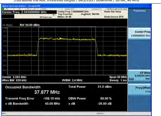
3 dB above the AGC threshold output / BRS/EBS / Downlink / 5G NR\_40 MHz
