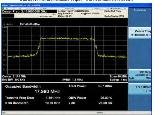
3 dB above the AGC threshold output / AWS / Downlink / LTE 20 MHz
