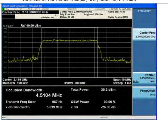
3 dB above the AGC threshold output / AWS / Downlink / LTE 5 MHz
