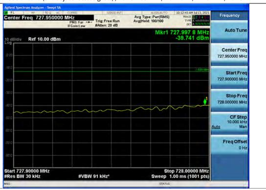
Out-of-band (two adjacent test signals) / Lower 700 MHz / Downlink / LTE 5 MHz / Upper
