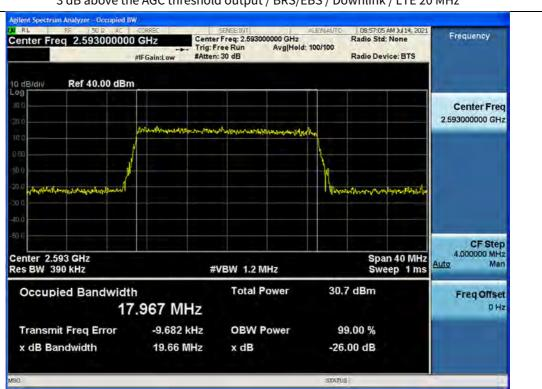
3 dB above the AGC threshold output / BRS/EBS / Downlink / LTE 20 MHz
