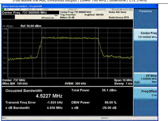
3 dB above the AGC threshold output / Lower 700 MHz / Downlink / LTE 5 MHz
