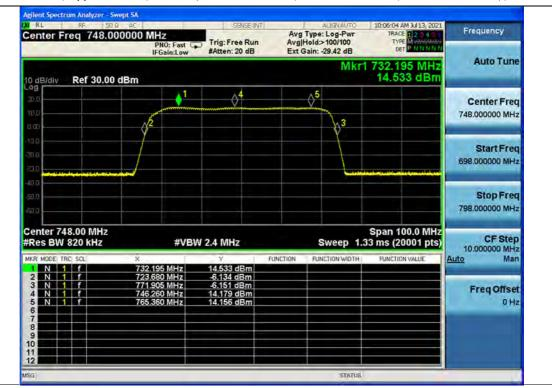
Lower 700 MHz / Upper 700 MHz / FirstNet (728 MHz ~ 746 MHz / 746 MHz ~ 757 MHz / 758 MHz ~ 768 MHz) / Downlink
