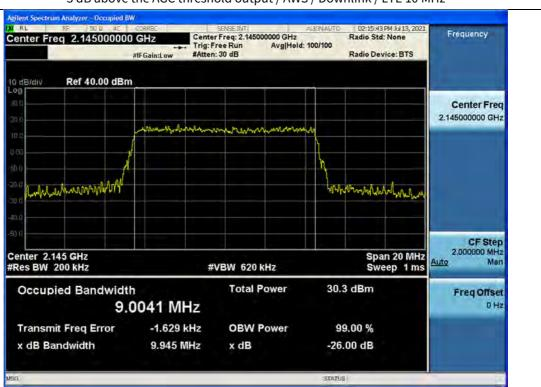
3 dB above the AGC threshold output / AWS / Downlink / LTE 10 MHz
