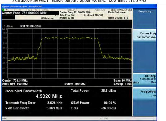
3 dB above the AGC threshold output / Upper 700 MHz / Downlink / LTE 5 MHz
