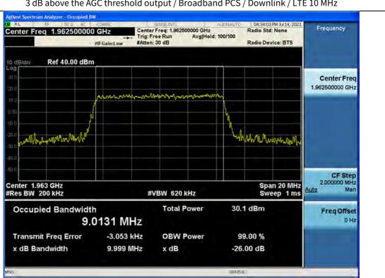
3 dB above the AGC threshold output / Broadband PCS / Downlink / LTE 10 MHz
