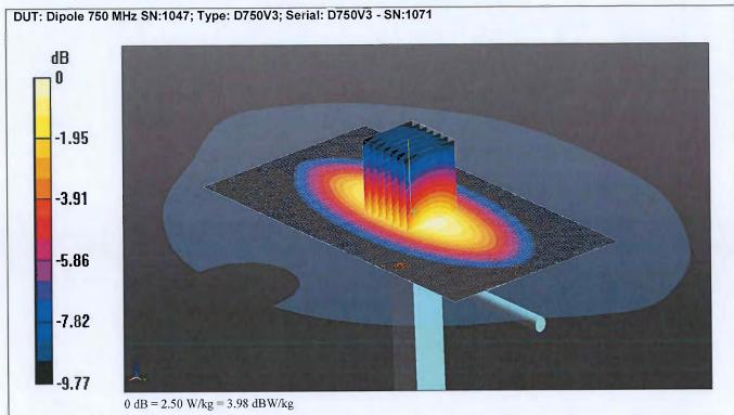
Communication System: UID 0, CW; Frequency: 750 MHz; Duty Cycle: 1:1 Medium: 750,835,900,1800,1900 MHz HSL Medium parameters used: f = 750 MHz;  $\sigma$  = 0.914 S/m;  $\epsilon_r$  = 41.936;  $\rho$  = 1000 kg/m<sup>3</sup> Phantom section: Flat Section
