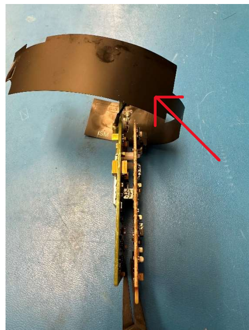
Side Profile (Cellular and ISM antenna)
