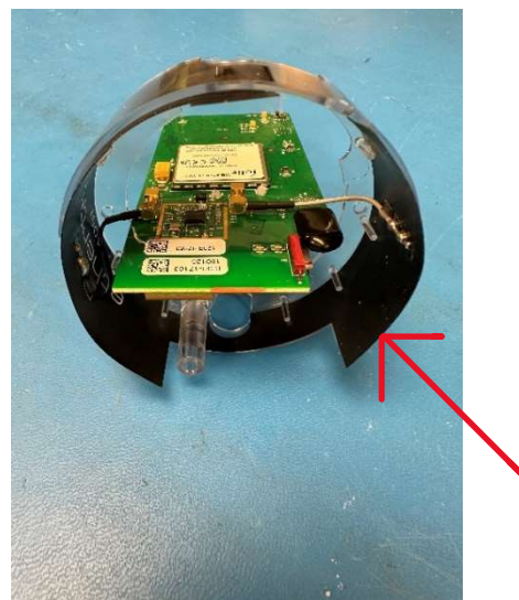
Top Internal View (Cellular and ISM antenna)
