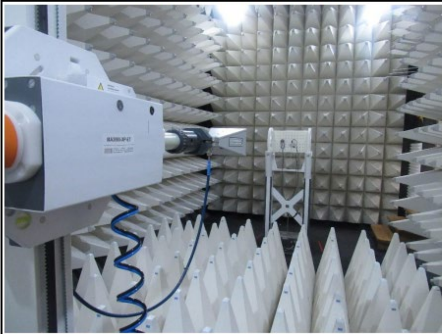
Setup for measurements above 1 GHz
