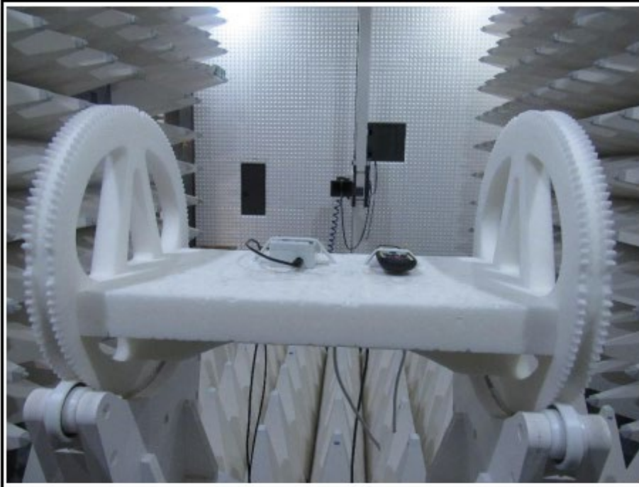
Setup for measurements above 1 GHz
