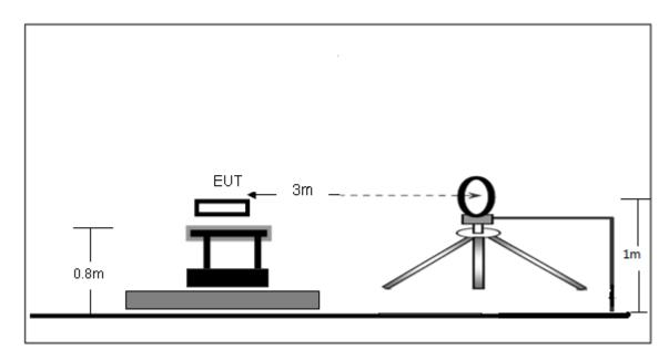
(B) Radiated Emission Test-Up Frequency 30MHz~1GHz
