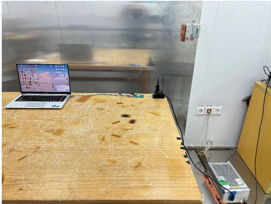
Photo of Setup for Radiated Emission (30MHz~1GHz)
