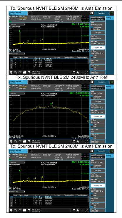
Note: The low frequency, which started from 9 kHz to 30 MHz, was pre-scanned and the result which was 20dB lower than the limit line was not reported.
