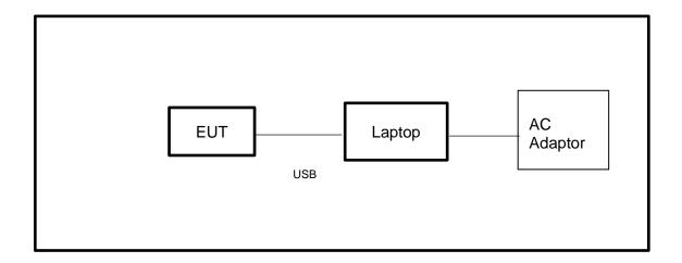
Note: AC Adaptor only use for AC POWER LINE CONDUCTED EMISSION test
