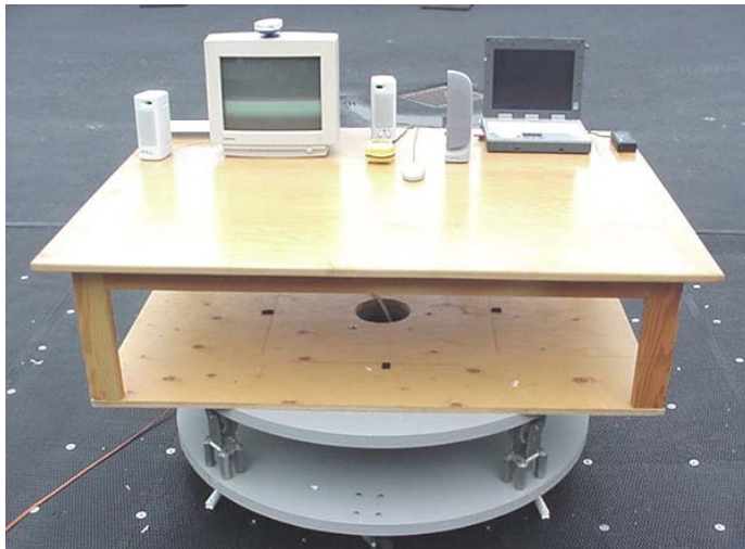
Photograph E-3 - Front of Radiated Emission Configuration
