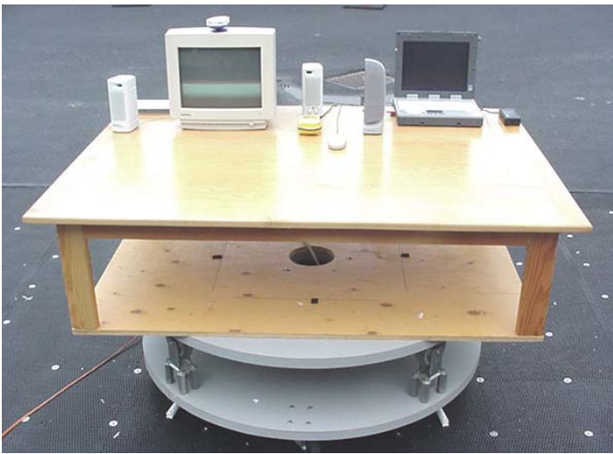
Photograph F-3 - Front of Radiated Emission Configuration
