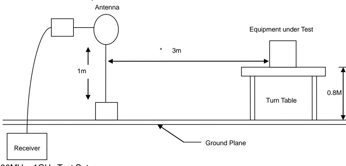
30MHz- 1GHz Test Setup
