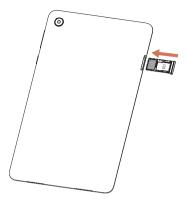
Open the slot and insert the SD card.
