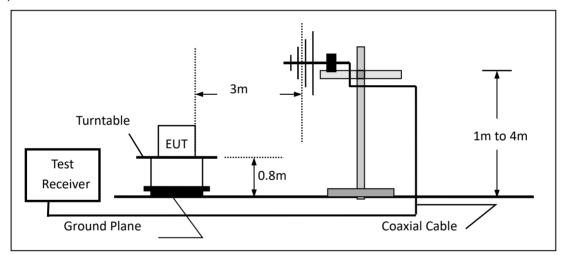
(c) For radiated emissions above 1000MHz
