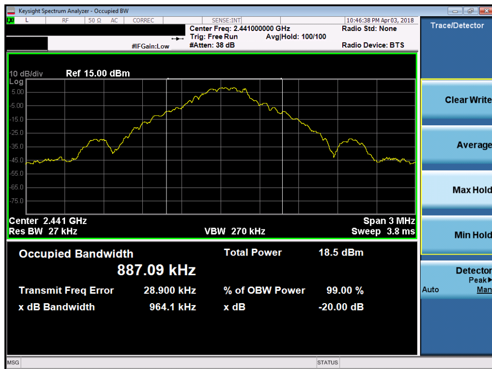
Plot 7-2. 20dB Bandwidth Plot (Bluetooth, 1Mbps – Ch. 39)
