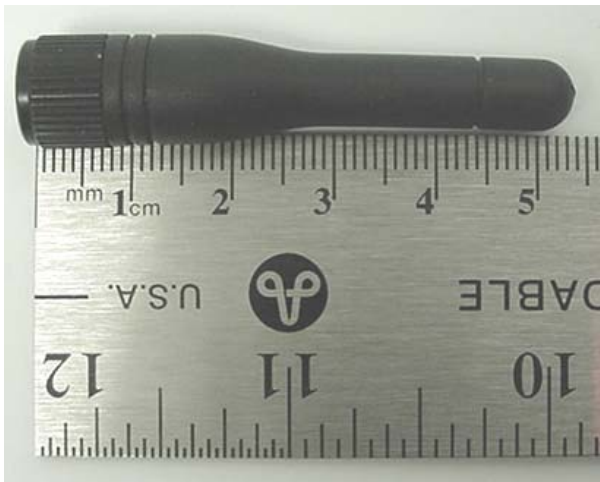
Dual-Band CDMA Antenna - Nearson 1/4-Wave Helix
