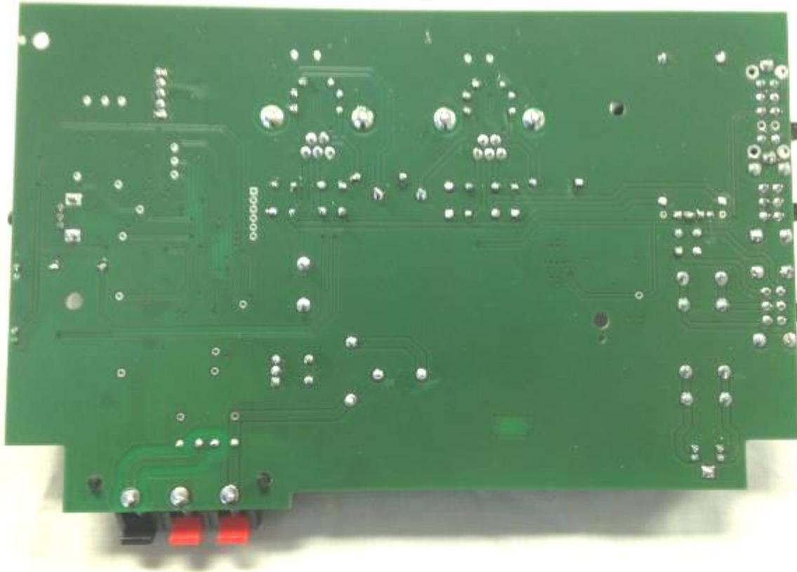
**Figure 3. PCB Solder Side**
