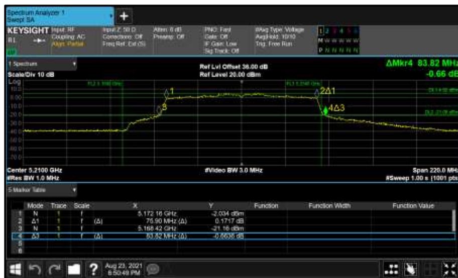
Figure 149 - Core 0 (A) 5210 MHz (CH42) 26 dB and 99% Bandwidth
