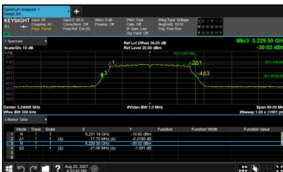
Figure 107 - Core 0 (A) 5240 MHz (CH48) 26 dB and 99% Bandwidth
