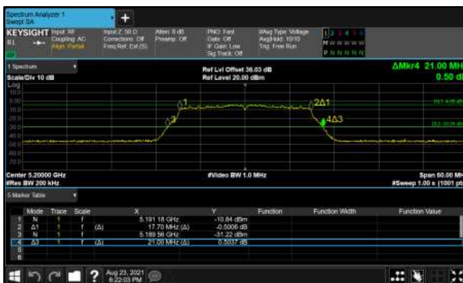
Figure 106 - Core 1 (B) 5200 MHz (CH40) 26 dB and 99% Bandwidth
