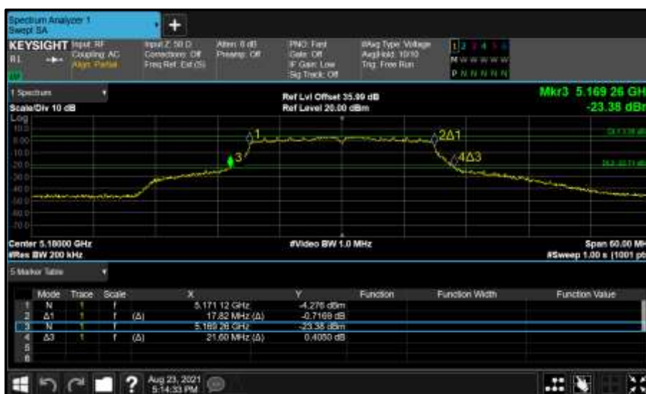
Figure 98 - Core 1 (B) 5180 MHz (CH36) 26 dB and 99% Bandwidth
