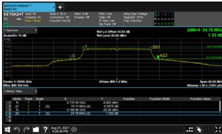
Figure 163 - Core 0 (A) 5180 MHz (CH36) 26 dB and 99% Bandwidth
