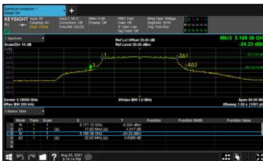
Figure 97 - Core 0 (A) 5180 MHz (CH36) 26 dB and 99% Bandwidth
