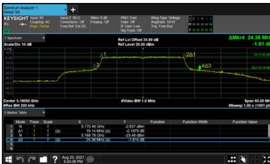
Figure 158 - Core 1 (B) 5180 MHz (CH36) 26 dB and 99% Bandwidth
