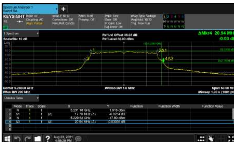
Figure 93 - Core 0 (A) 5240 MHz (CH48) 26 dB and 99% Bandwidth
