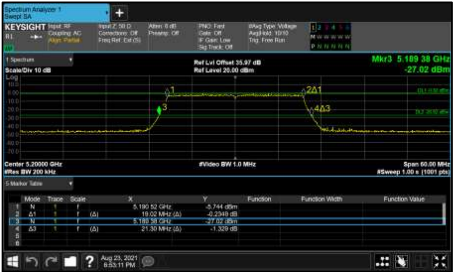
Figure 177 - Core 0 (A) 5200 MHz (CH40) 26 dB and 99% Bandwidth
