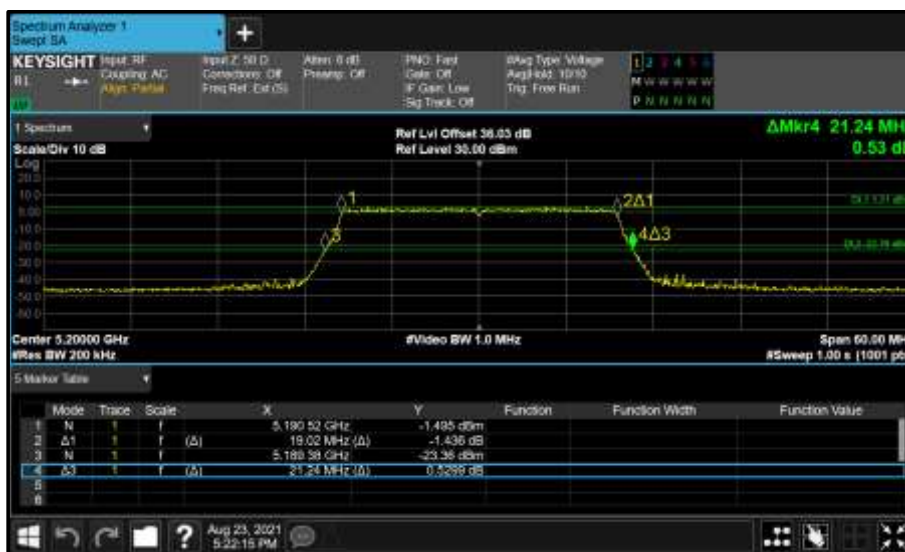
Figure 160 - Core 1 (B) 5200 MHz (CH40) 26 dB and 99% Bandwidth
