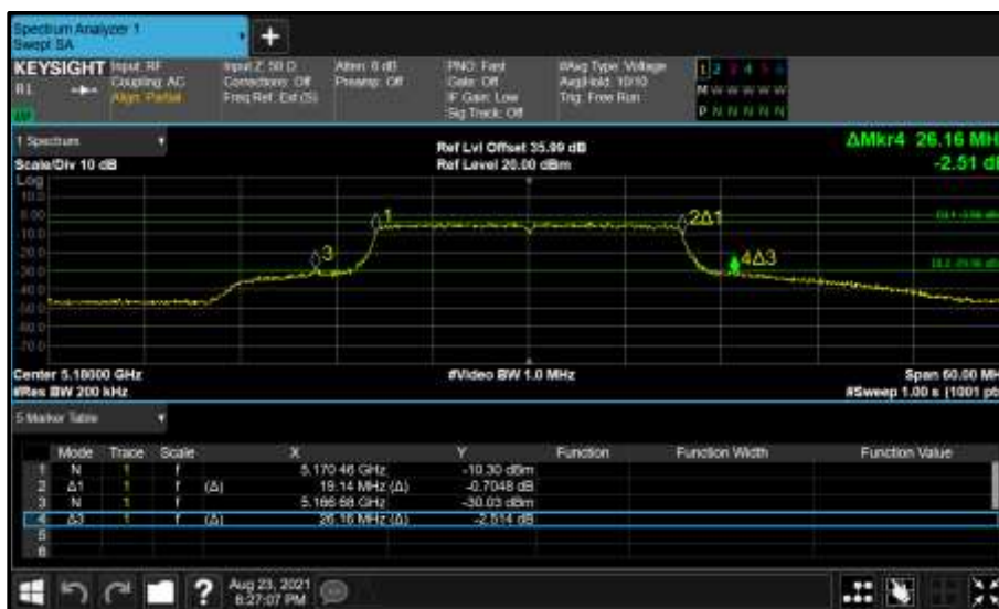
Figure 164 - Core 1 (B) 5180 MHz (CH36) 26 dB and 99% Bandwidth
