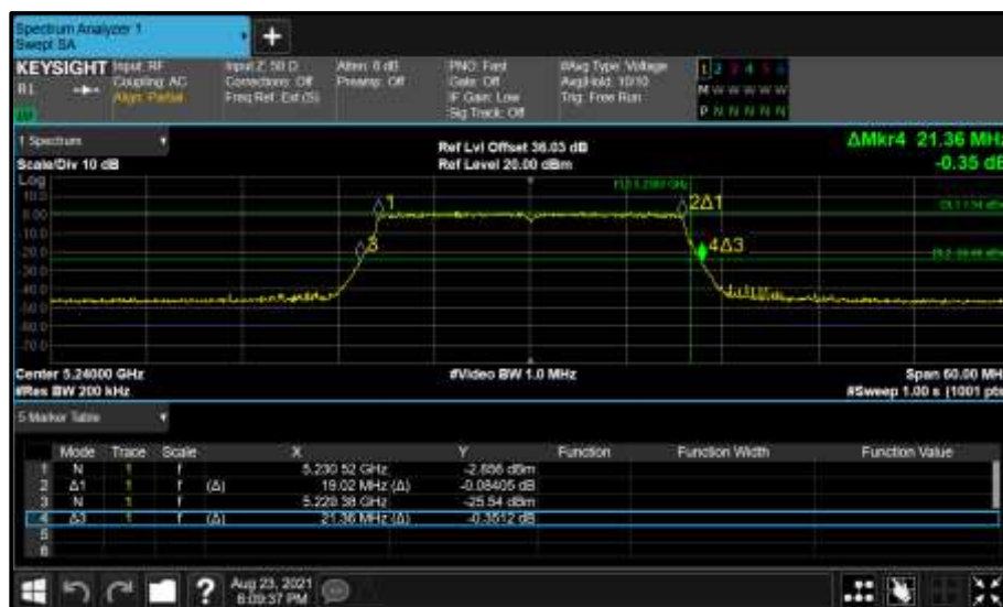
Figure 156 - Core 0 (A) 5240 MHz (CH48) 26 dB and 99% Bandwidth
