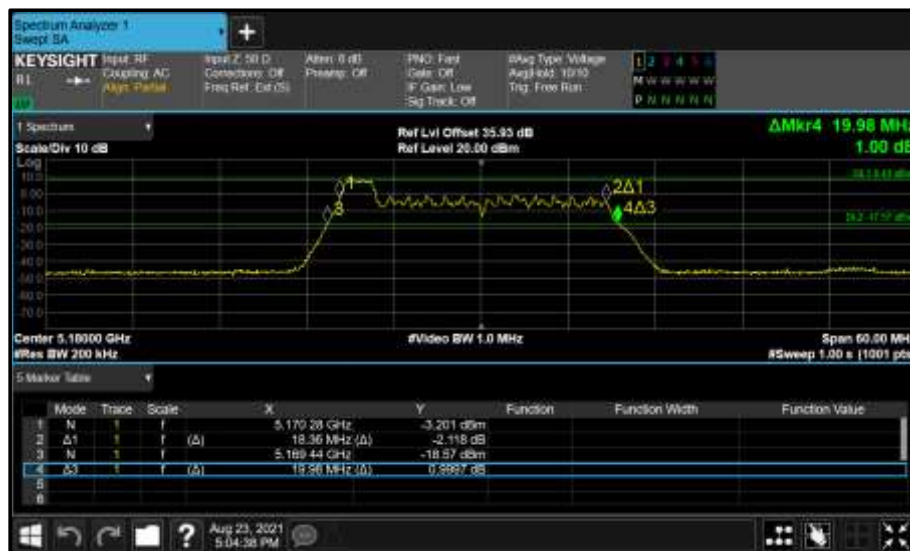
Figure 181 - Core 0 (A) 5180 MHz (CH36) 26 dB and 99% Bandwidth
