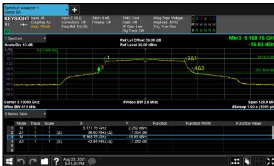
Figure 134 - Core 1 (B) 5190 MHz (CH38) 26 dB and 99% Bandwidth
