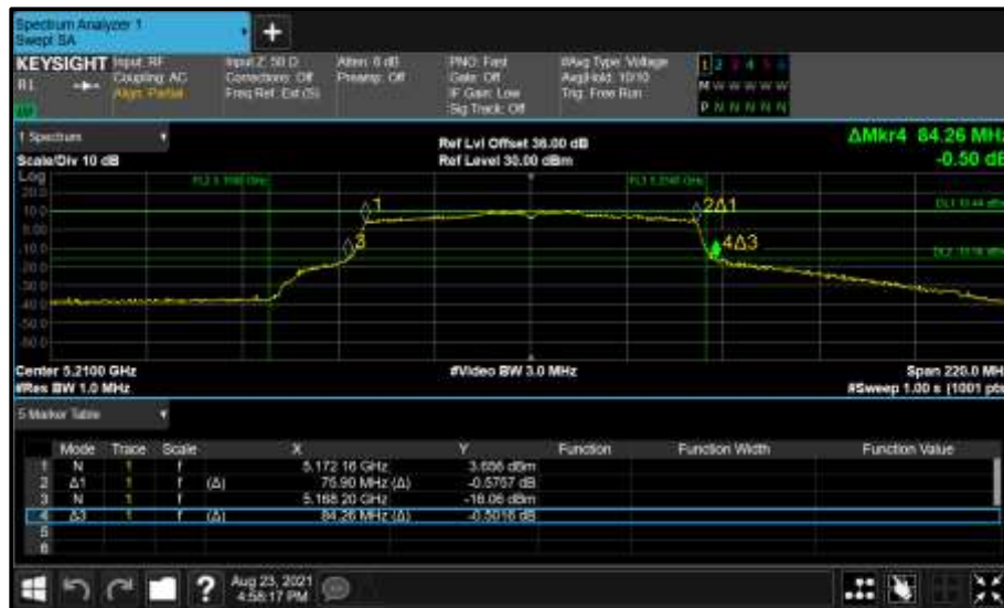
Figure 141 - Core 0 (A) 5210 MHz (CH42) 26 dB and 99% Bandwidth
