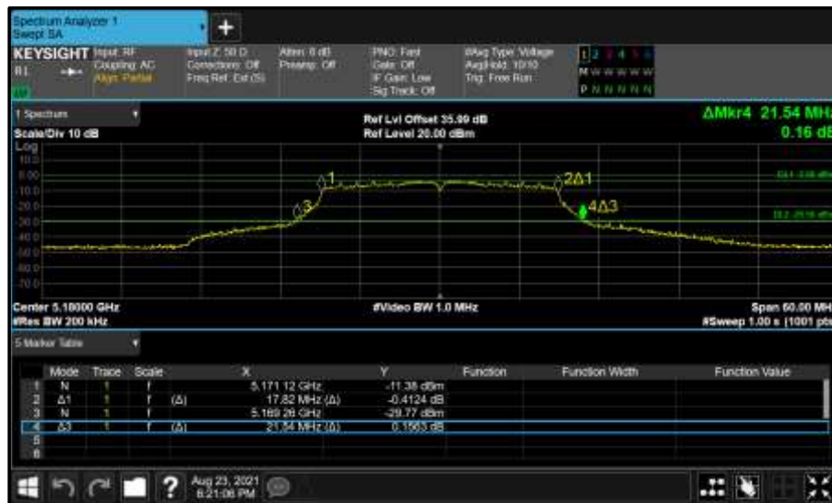
Figure 104 - Core 1 (B) 5180 MHz (CH36) 26 dB and 99% Bandwidth
