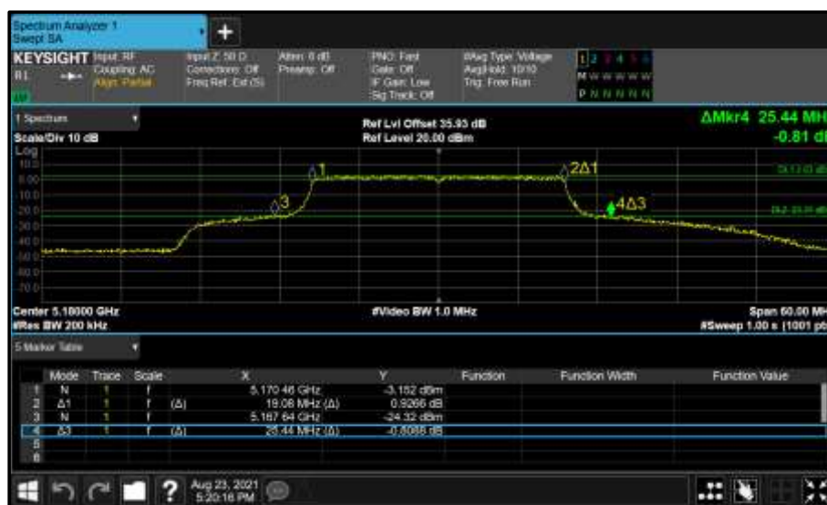
Figure 157 - Core 0 (A) 5180 MHz (CH36) 26 dB and 99% Bandwidth
