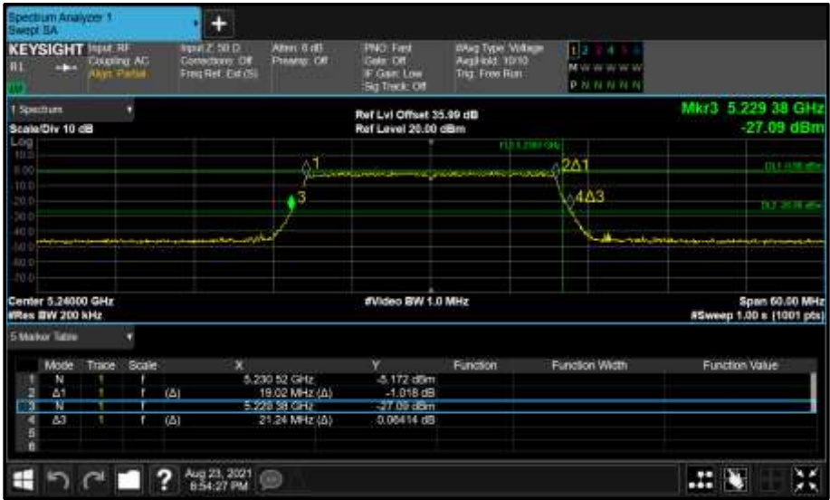
Figure 180 - Core 1 (B) 5240 MHz (CH48) 26 dB and 99% Bandwidth
