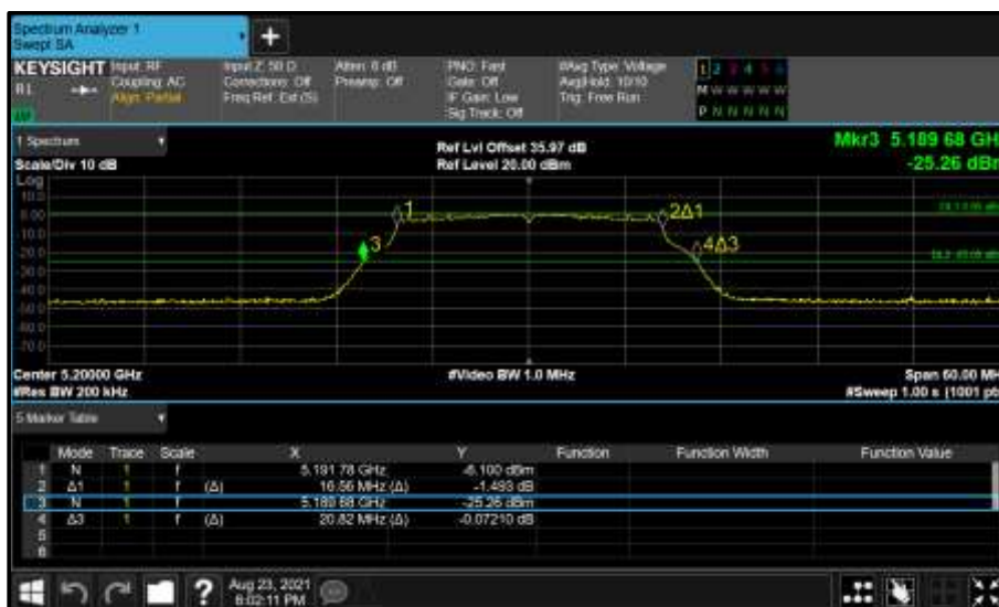
Figure 89 - Core 0 (A) 5200 MHz (CH40) 26 dB and 99% Bandwidth
