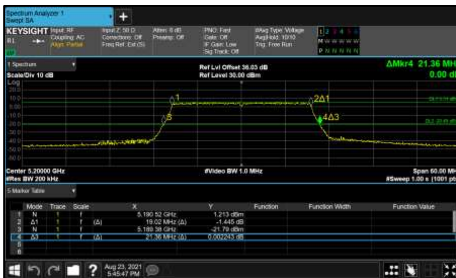
Figure 172 - Core 1 (B) 5200 MHz (CH40) 26 dB and 99% Bandwidth
