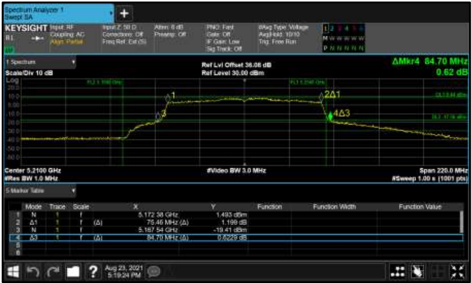
Figure 144 - Core 1 (B) 5210 MHz (CH42) 26 dB and 99% Bandwidth
