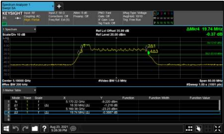
Figure 188 - Core 1 (B) 5180 MHz (CH36) 26 dB and 99% Bandwidth
