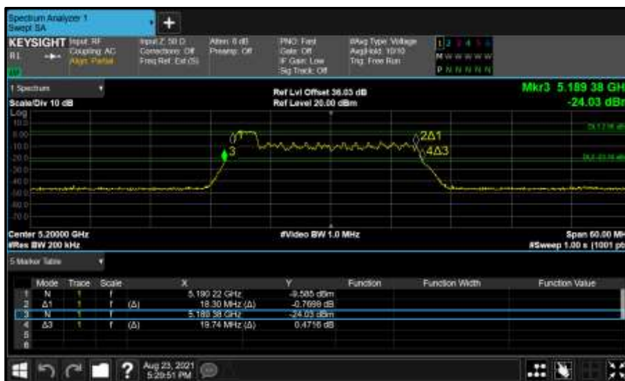
Figure 190 - Core 1 (B) 5200 MHz (CH40) 26 dB and 99% Bandwidth
