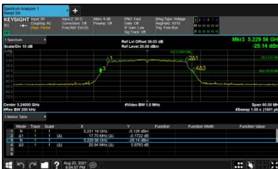
Figure 96 - Core 0 (A) 5240 MHz (CH48) 26 dB and 99% Bandwidth
