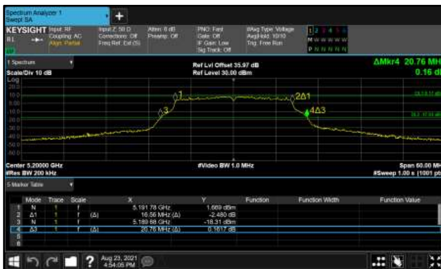
Figure 86 - Core 0 (A) 5200 MHz (CH40) 26 dB and 99% Bandwidth
