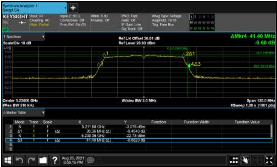
Figure 140 - Core 1 (B) 5230 MHz (CH46) 26 dB and 99% Bandwidth
