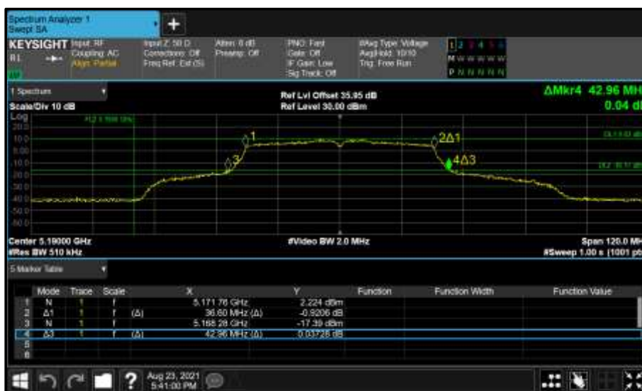
Figure 133 - Core 0 (A) 5190 MHz (CH38) 26 dB and 99% Bandwidth
