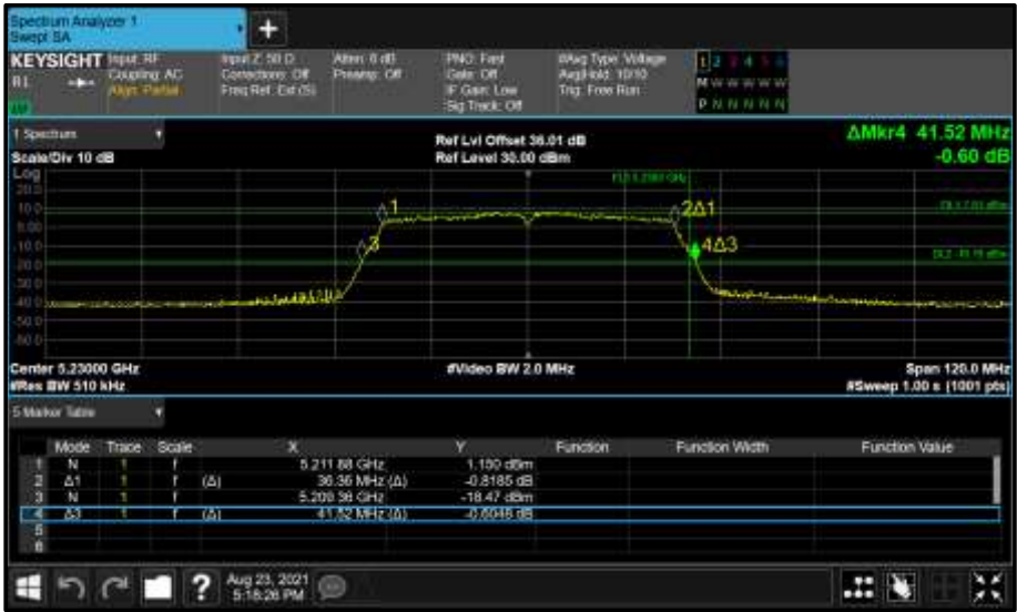
Figure 128 - Core 1 (B) 5230 MHz (CH46) 26 dB and 99% Bandwidth
