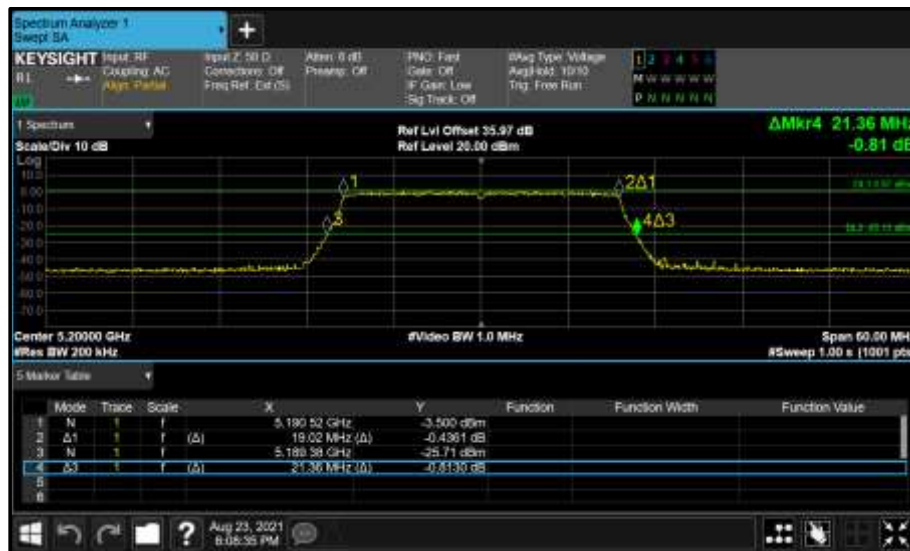
Figure 155 - Core 0 (A) 5200 MHz (CH40) 26 dB and 99% Bandwidth
