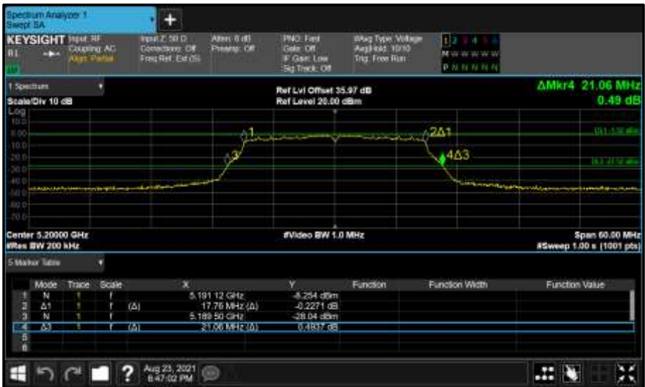
Figure 117 - Core 0 (A) 5200 MHz (CH40) 26 dB and 99% Bandwidth
