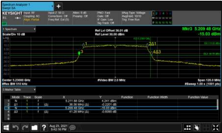
Figure 136 - Core 1 (B) 5230 MHz (CH46) 26 dB and 99% Bandwidth
