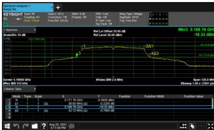
Figure 125 - Core 0 (A) 5190 MHz (CH38) 26 dB and 99% Bandwidth
