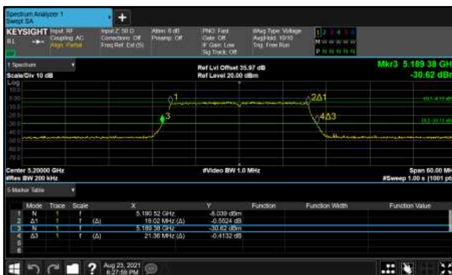
Figure 165 - Core 0 (A) 5200 MHz (CH40) 26 dB and 99% Bandwidth
