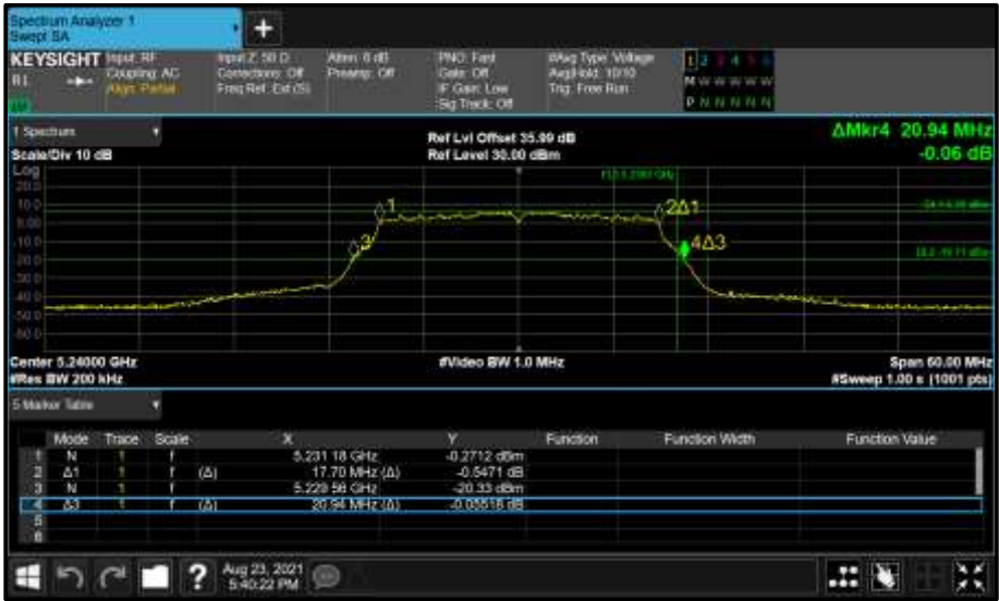
Figure 114 - Core 1 (B) 5240 MHz (CH48) 26 dB and 99% Bandwidth
