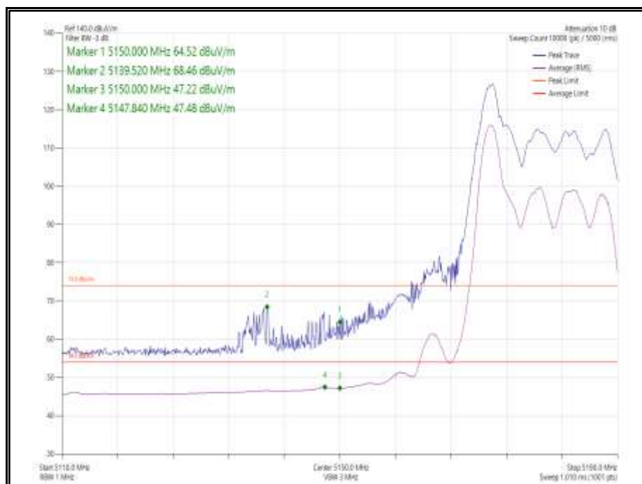
Figure 18 - 802.11ax HE20 SDM, Cores 0-1, 26-0 - 5180 MHz Band Edge Frequency 5150 MHz
