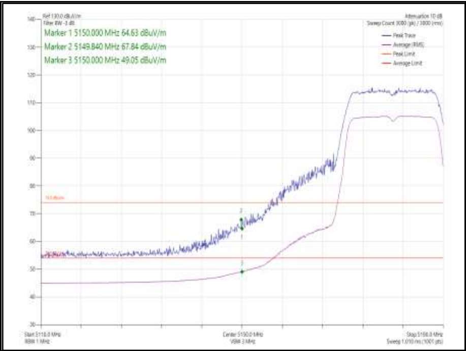
Figure 2 - 802.11n HT20, Core 0 - 5180 MHz, Band Edge Frequency 5150 MHz
