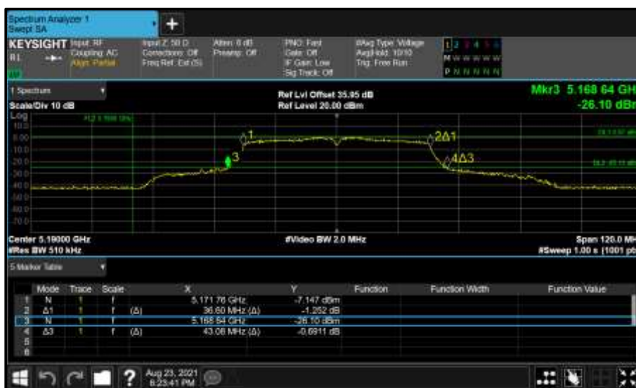
Figure 129 - Core 0 (A) 5190 MHz (CH38) 26 dB and 99% Bandwidth
