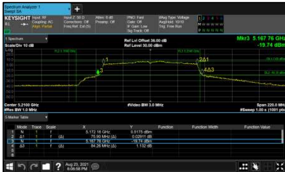
Figure 142 - Core 0 (A) 5210 MHz (CH42) 26 dB and 99% Bandwidth
