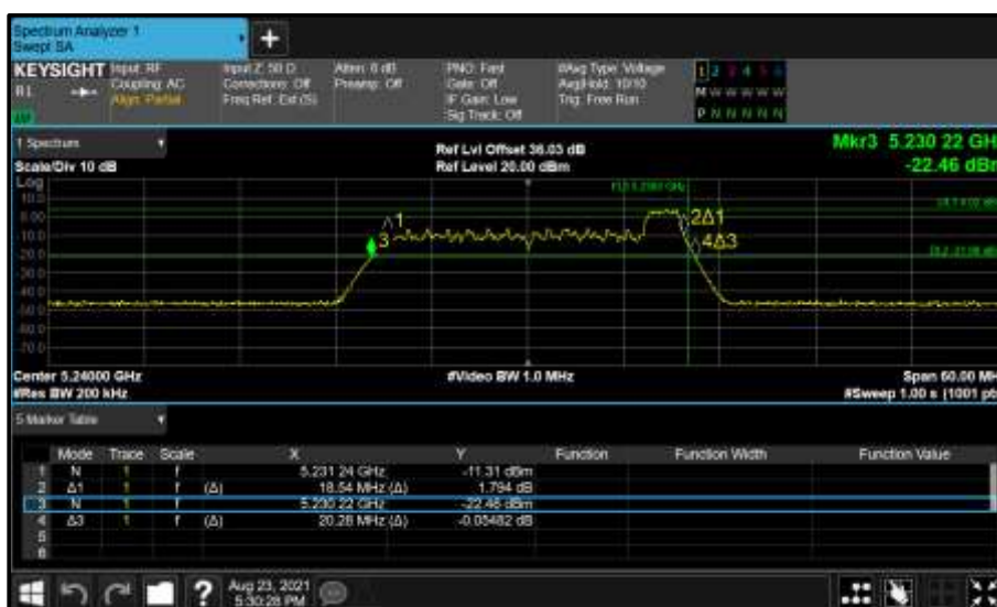
Figure 191 - Core 0 (A) 5240 MHz (CH48) 26 dB and 99% Bandwidth
