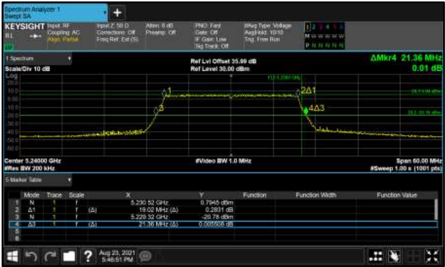
Figure 174 - Core 1 (B) 5240 MHz (CH48) 26 dB and 99% Bandwidth
