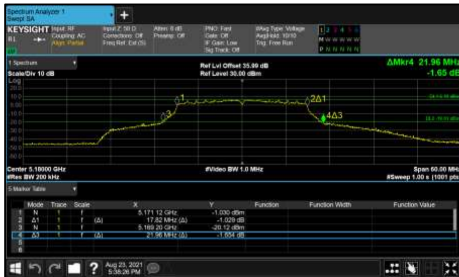
Figure 110 - Core 1 (B) 5180 MHz (CH36) 26 dB and 99% Bandwidth
