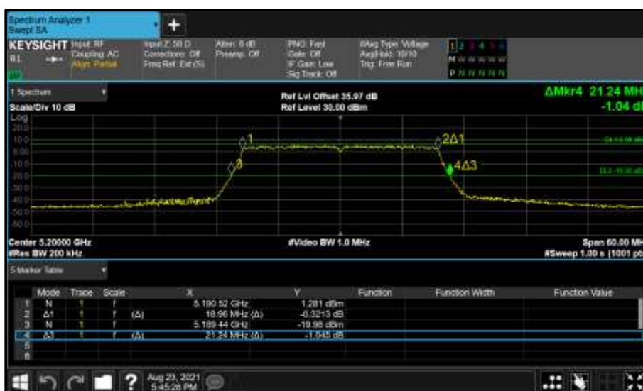
Figure 171 - Core 0 (A) 5200 MHz (CH40) 26 dB and 99% Bandwidth
