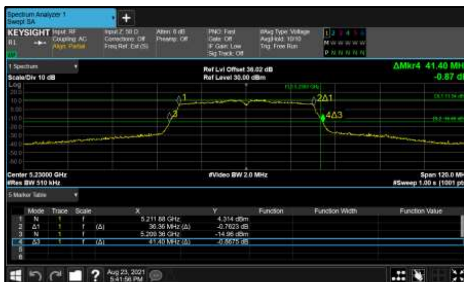
Figure 135 - Core 0 (A) 5230 MHz (CH46) 26 dB and 99% Bandwidth
