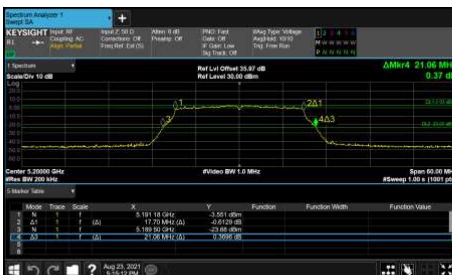
Figure 99 - Core 0 (A) 5200 MHz (CH40) 26 dB and 99% Bandwidth
