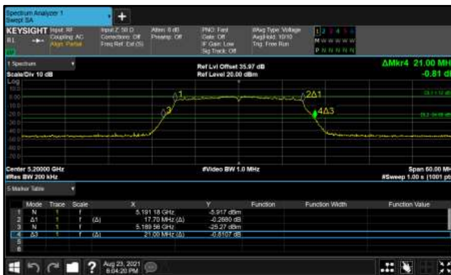
Figure 95 - Core 0 (A) 5200 MHz (CH40) 26 dB and 99% Bandwidth
