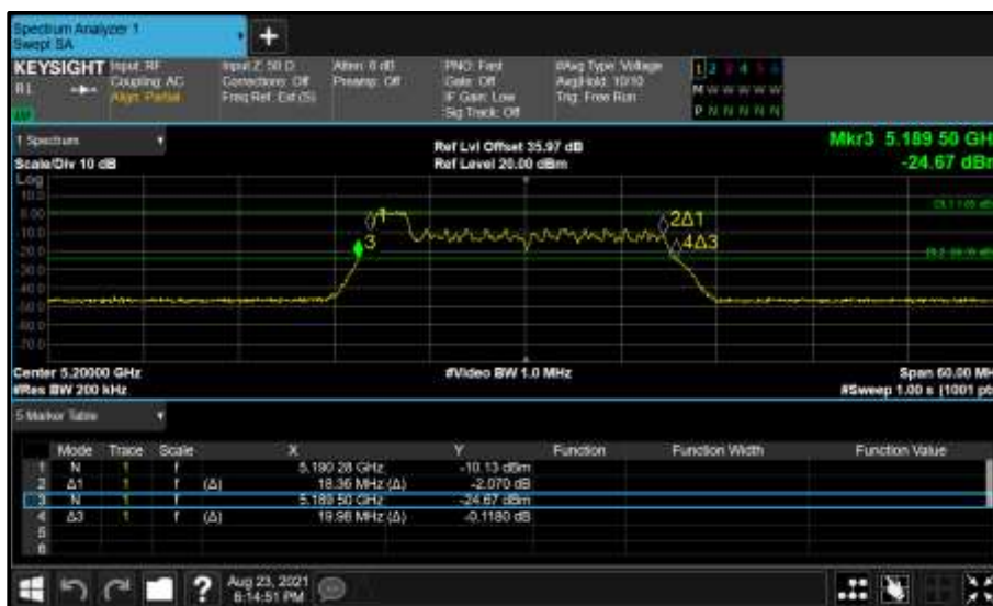
Figure 185 - Core 0 (A) 5200 MHz (CH40) 26 dB and 99% Bandwidth
