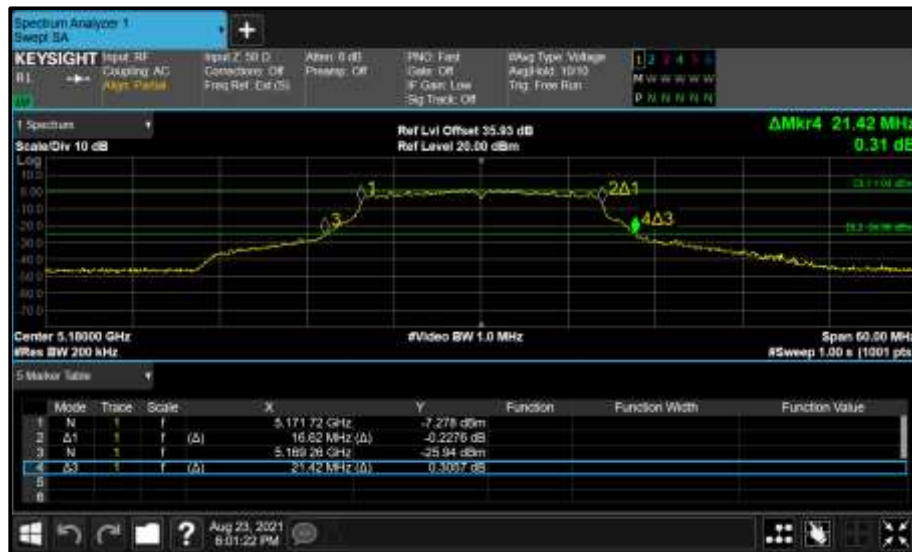
Figure 88 - Core 0 (A) 5180 MHz (CH36) 26 dB and 99% Bandwidth
