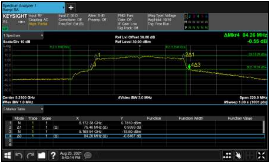
Figure 148 - Core 1 (B) 5210 MHz (CH42) 26 dB and 99% Bandwidth
