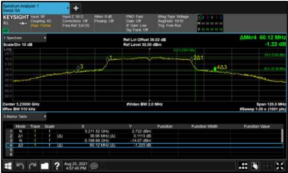
Figure 122 - Core 0 (A) 5230 MHz (CH46) 26 dB and 99% Bandwidth
