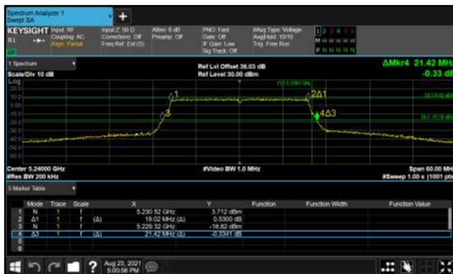
Figure 153 - Core 0 (A) 5240 MHz (CH48) 26 dB and 99% Bandwidth
