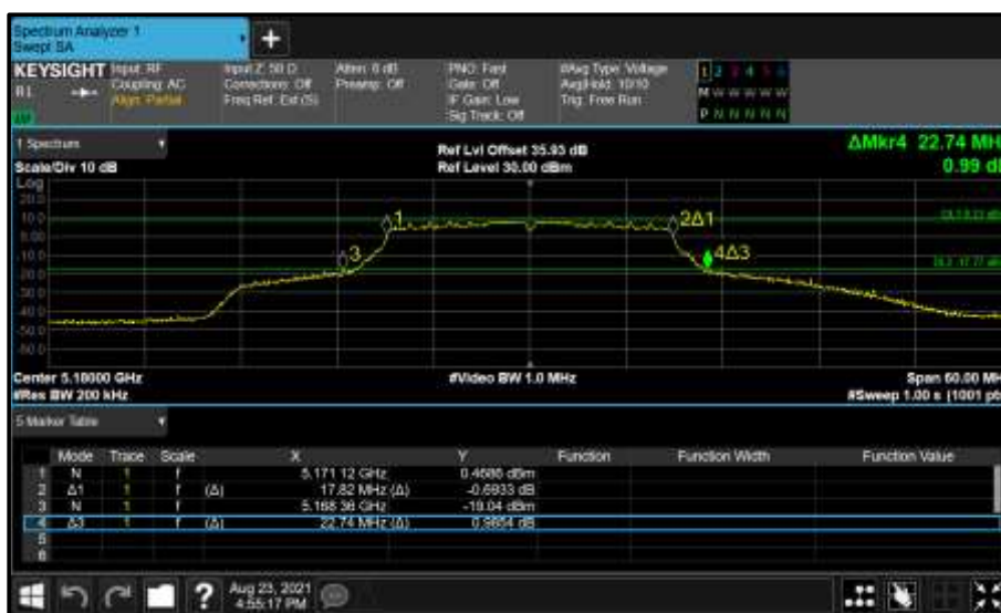
Figure 91 - Core 0 (A) 5180 MHz (CH36) 26 dB and 99% Bandwidth
