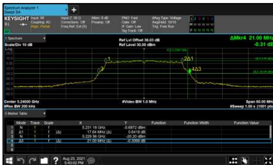
Figure 113 - Core 0 (A) 5240 MHz (CH48) 26 dB and 99% Bandwidth
