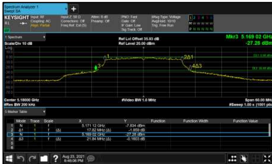
Figure 115 - Core 0 (A) 5180 MHz (CH36) 26 dB and 99% Bandwidth
