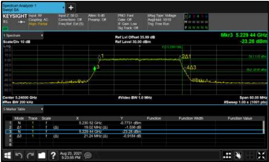
Figure 162 - Core 1 (B) 5240 MHz (CH48) 26 dB and 99% Bandwidth
