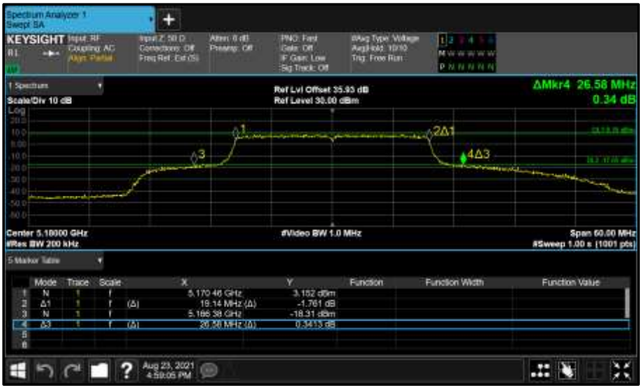
Figure 151 - Core 0 (A) 5180 MHz (CH36) 26 dB and 99% Bandwidth
