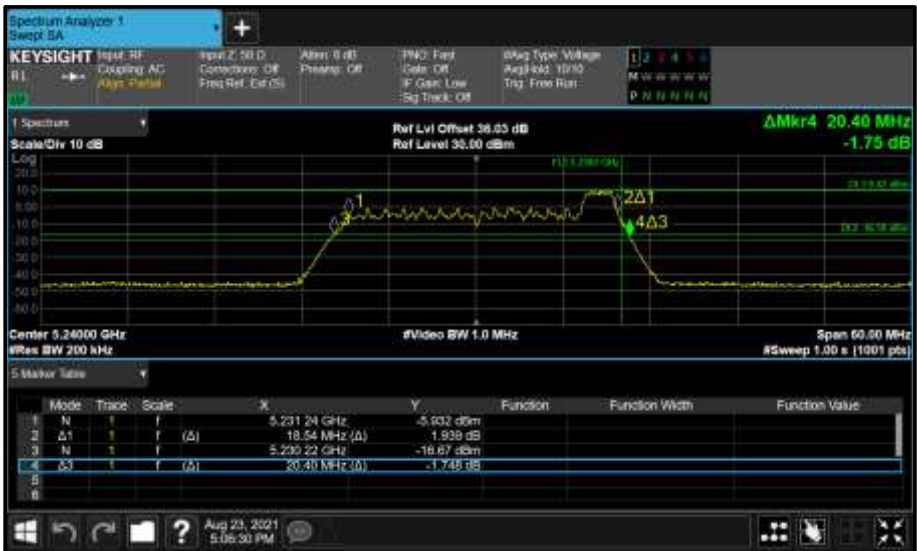
Figure 183 - Core 0 (A) 5240 MHz (CH48) 26 dB and 99% Bandwidth
