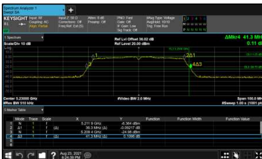
Figure 131 - Core 0 (A) 5230 MHz (CH46) 26 dB and 99% Bandwidth
