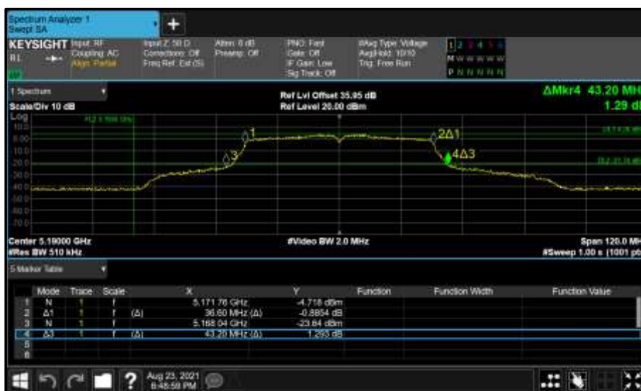
Figure 137 - Core 0 (A) 5190 MHz (CH38) 26 dB and 99% Bandwidth
