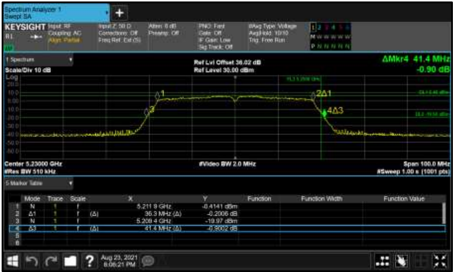
Figure 124 - Core 0 (A) 5230 MHz (CH46) 26 dB and 99% Bandwidth
