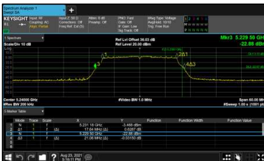
Figure 101 - Core 0 (A) 5240 MHz (CH48) 26 dB and 99% Bandwidth
