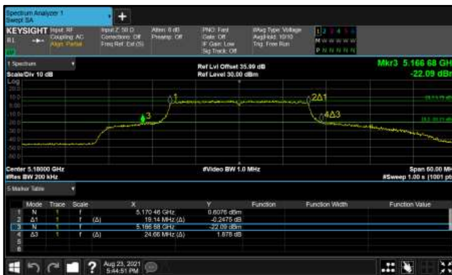
Figure 170 - Core 1 (B) 5180 MHz (CH36) 26 dB and 99% Bandwidth
