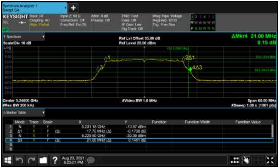
Figure 108 - Core 1 (B) 5240 MHz (CH48) 26 dB and 99% Bandwidth
