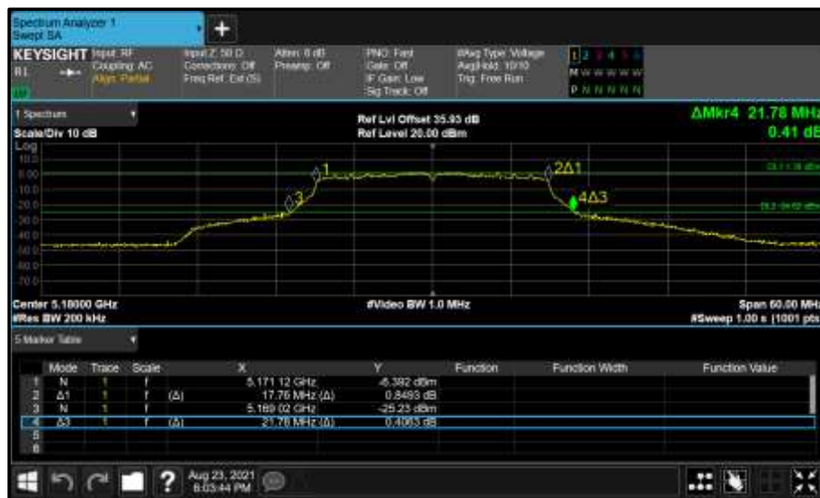
Figure 94 - Core 0 (A) 5180 MHz (CH36) 26 dB and 99% Bandwidth
