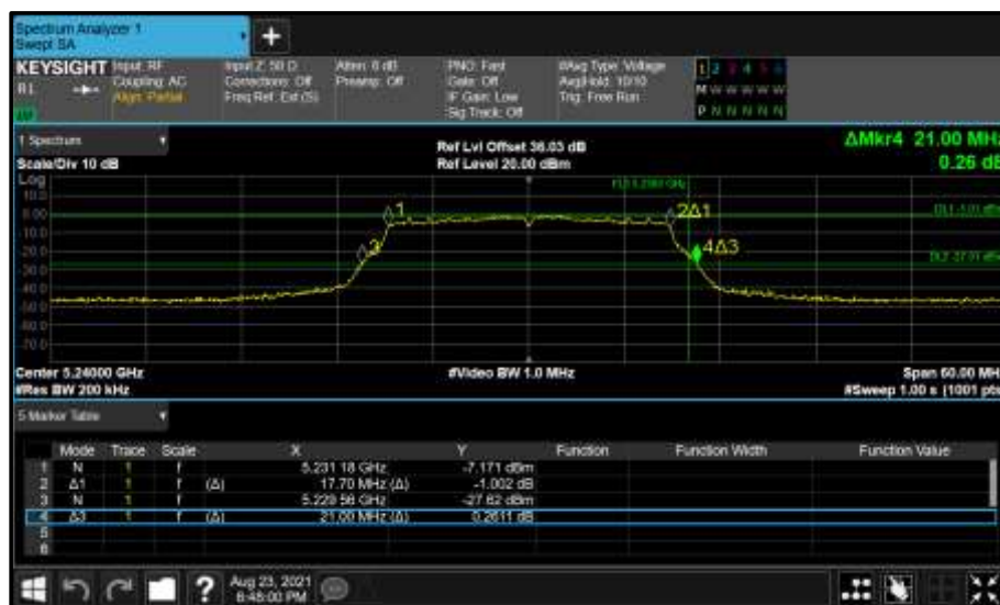
Figure 119 - Core 0 (A) 5240 MHz (CH48) 26 dB and 99% Bandwidth
