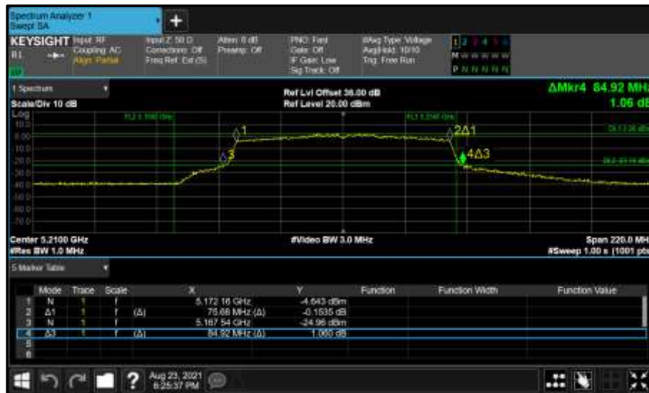
Figure 145 - Core 0 (A) 5210 MHz (CH42) 26 dB and 99% Bandwidth
