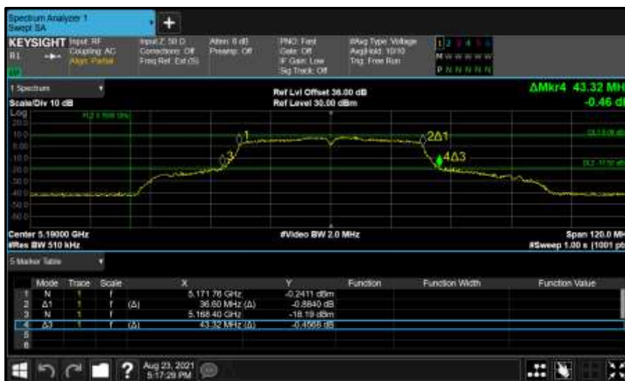
Figure 126 - Core 1 (B) 5190 MHz (CH38) 26 dB and 99% Bandwidth
