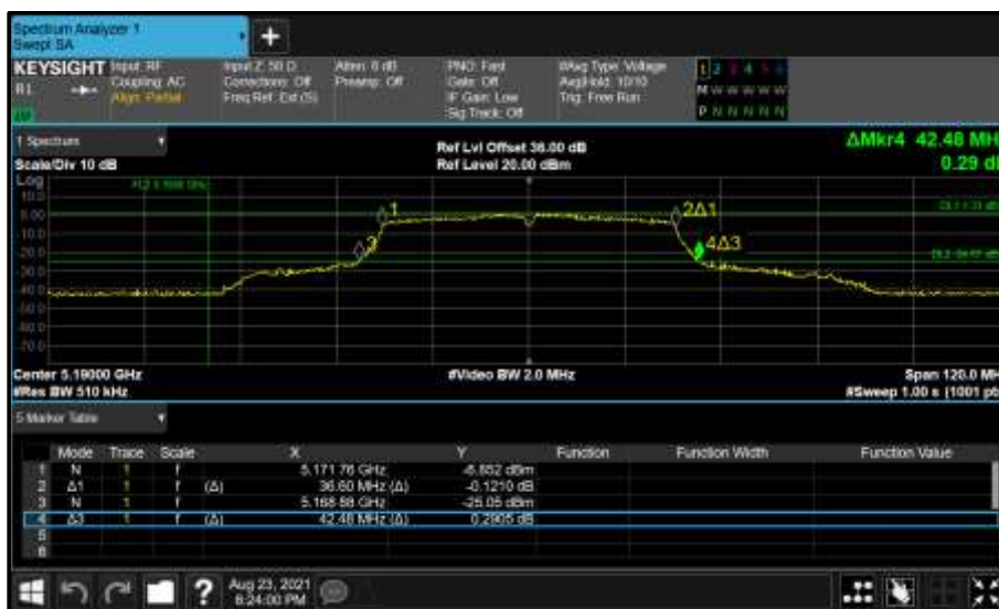
Figure 130 - Core 1 (B) 5190 MHz (CH38) 26 dB and 99% Bandwidth
