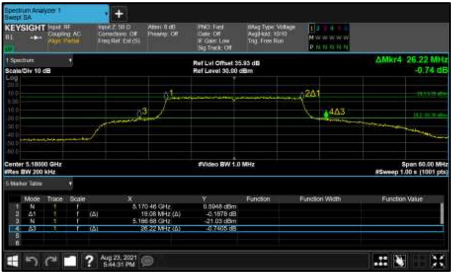
Figure 169 - Core 0 (A) 5180 MHz (CH36) 26 dB and 99% Bandwidth
