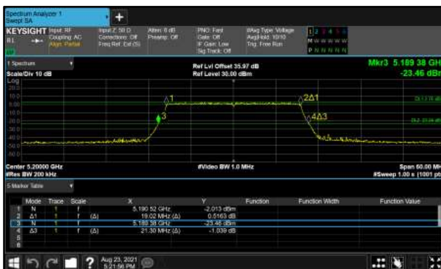
Figure 159 - Core 0 (A) 5200 MHz (CH40) 26 dB and 99% Bandwidth
