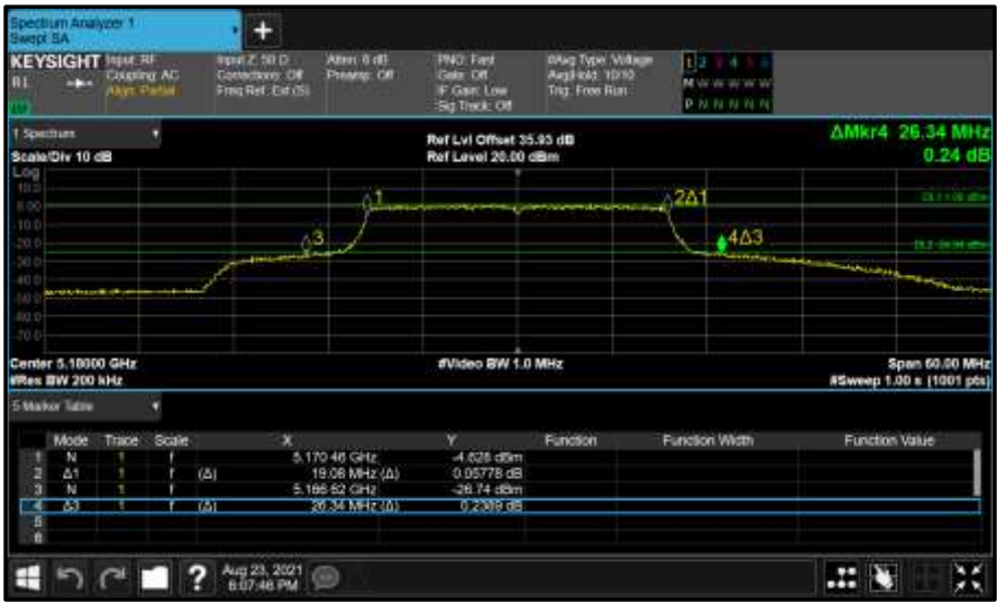
Figure 154 - Core 0 (A) 5180 MHz (CH36) 26 dB and 99% Bandwidth
