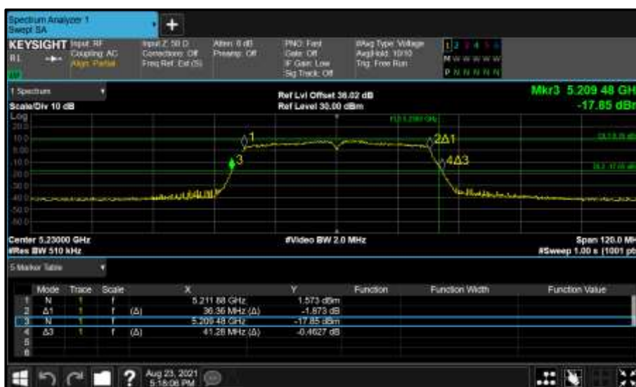
Figure 127 - Core 0 (A) 5230 MHz (CH46) 26 dB and 99% Bandwidth
