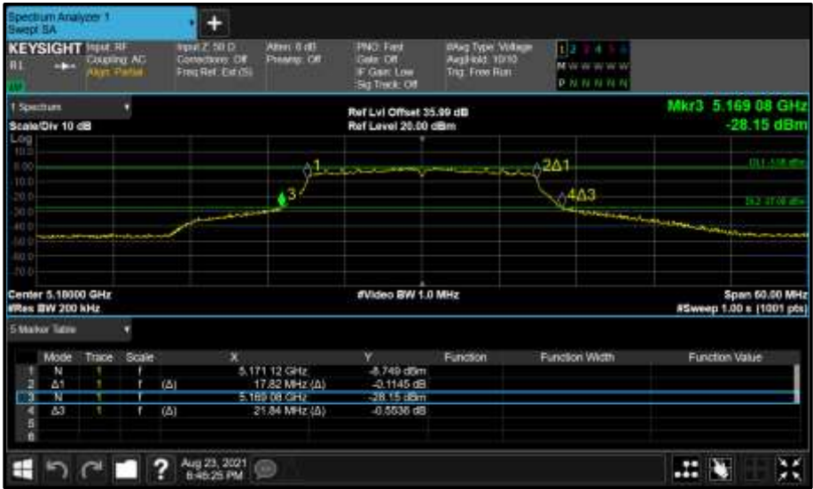
Figure 116 - Core 1 (B) 5180 MHz (CH36) 26 dB and 99% Bandwidth
