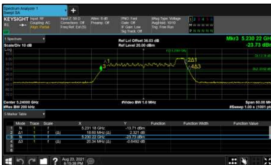
Figure 186 - Core 0 (A) 5240 MHz (CH48) 26 dB and 99% Bandwidth
