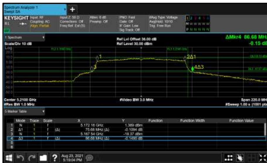
Figure 143 - Core 0 (A) 5210 MHz (CH42) 26 dB and 99% Bandwidth
