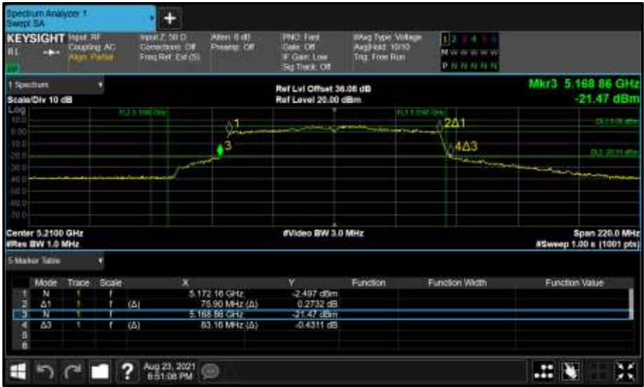
Figure 150 - Core 1 (B) 5210 MHz (CH42) 26 dB and 99% Bandwidth
