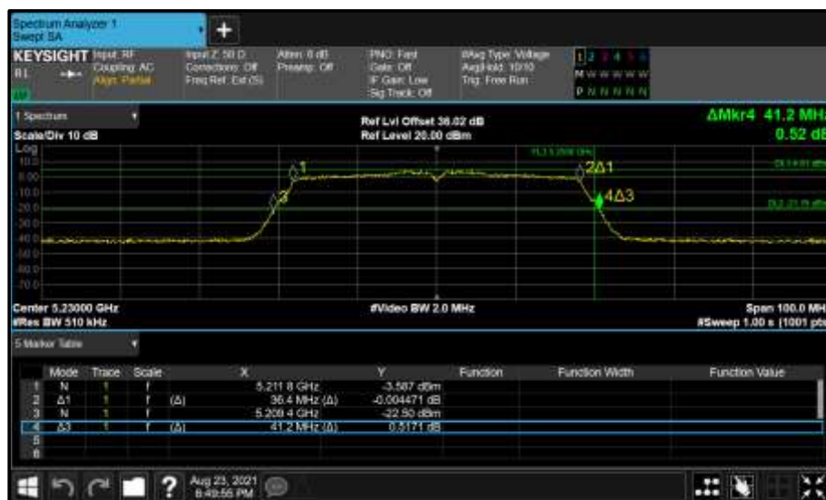
Figure 139 - Core 0 (A) 5230 MHz (CH46) 26 dB and 99% Bandwidth
