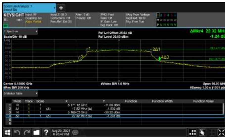
Figure 103 - Core 0 (A) 5180 MHz (CH36) 26 dB and 99% Bandwidth
