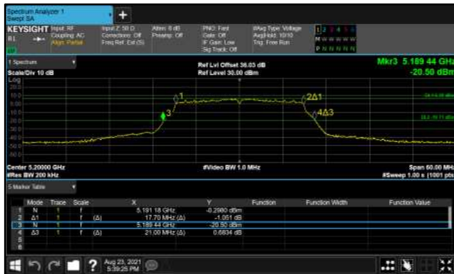
Figure 112 - Core 1 (B) 5200 MHz (CH40) 26 dB and 99% Bandwidth
