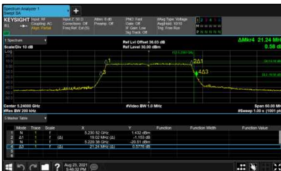
Figure 173 - Core 0 (A) 5240 MHz (CH48) 26 dB and 99% Bandwidth
