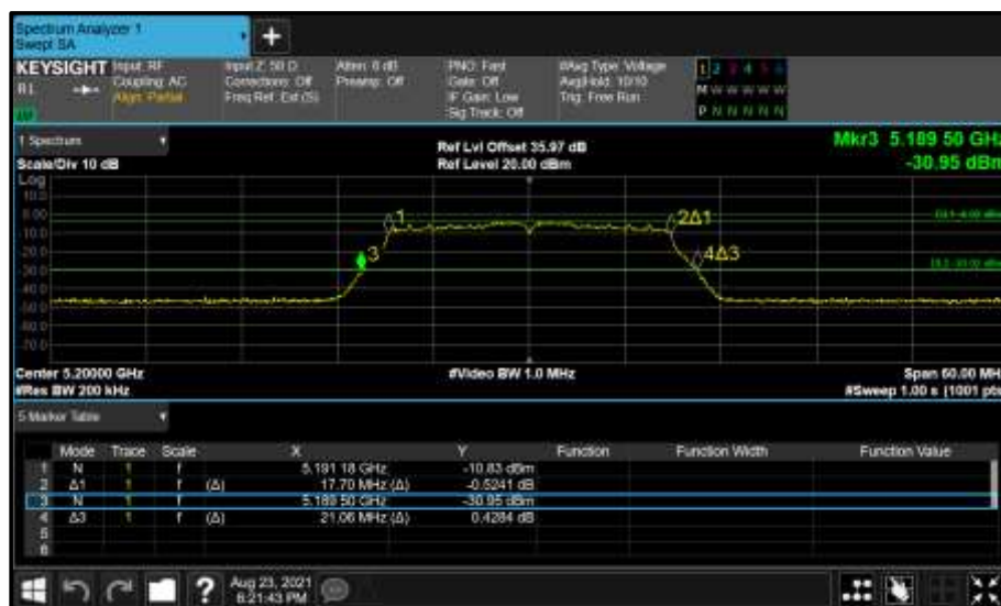
Figure 105 - Core 0 (A) 5200 MHz (CH40) 26 dB and 99% Bandwidth
