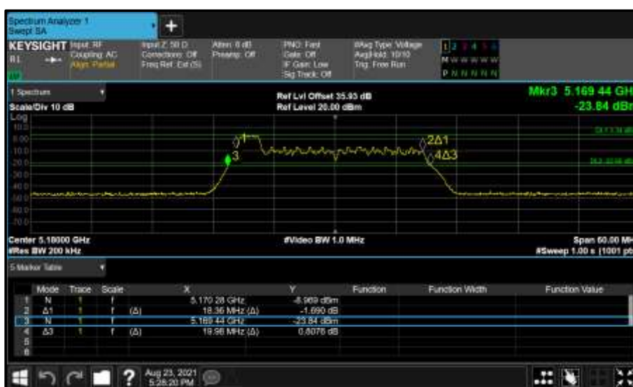
Figure 187 - Core 0 (A) 5180 MHz (CH36) 26 dB and 99% Bandwidth
