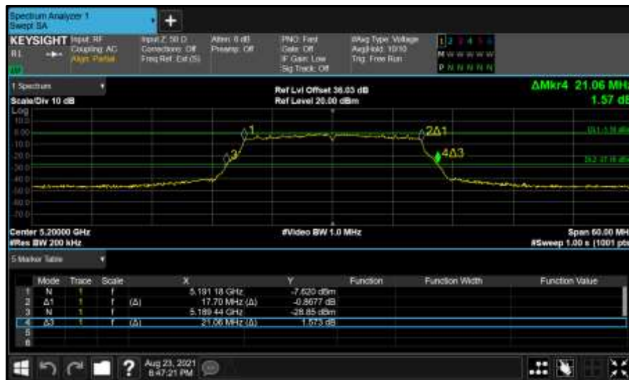
Figure 118 - Core 1 (B) 5200 MHz (CH40) 26 dB and 99% Bandwidth
