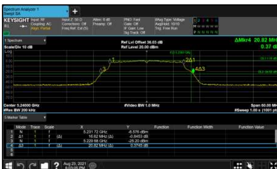
Figure 90 - Core 0 (A) 5240 MHz (CH48) 26 dB and 99% Bandwidth
