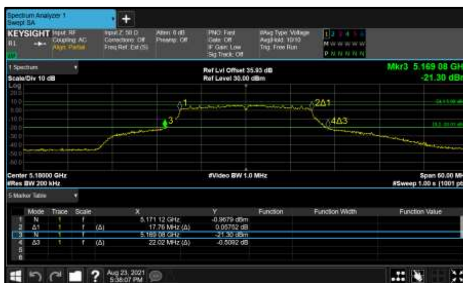
Figure 109 - Core 0 (A) 5180 MHz (CH36) 26 dB and 99% Bandwidth
