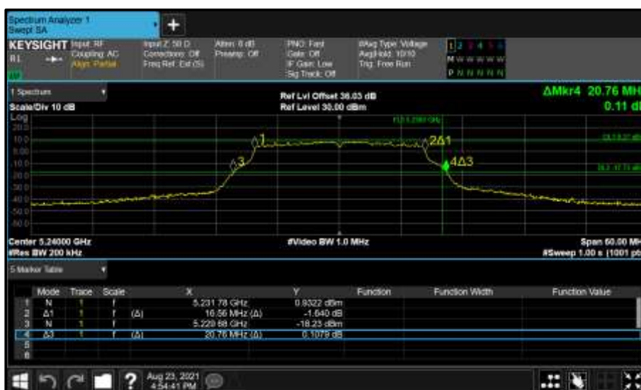
Figure 87 - Core 0 (A) 5240 MHz (CH48) 26 dB and 99% Bandwidth
