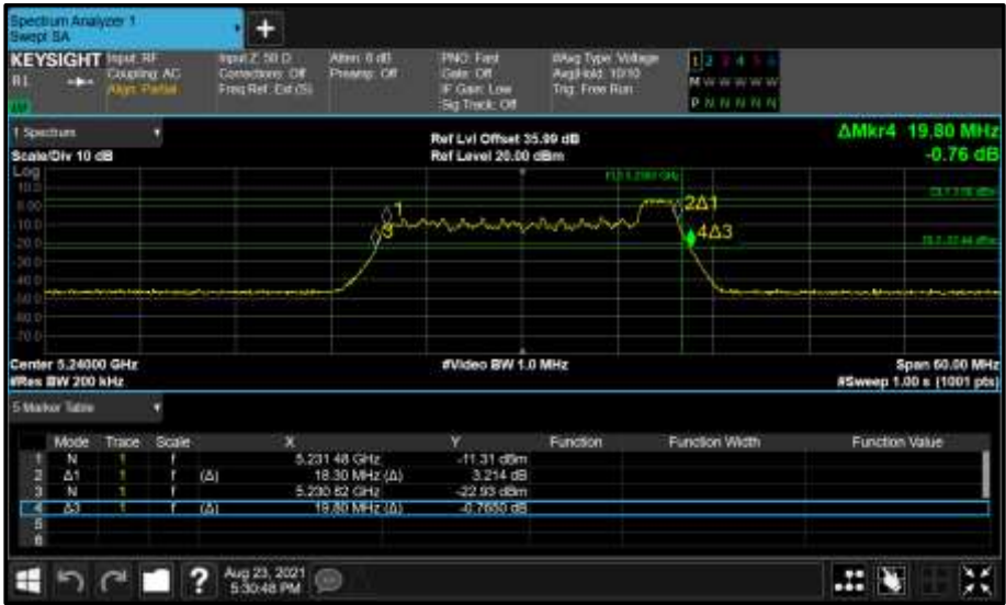
Figure 192 - Core 1 (B) 5240 MHz (CH48) 26 dB and 99% Bandwidth
