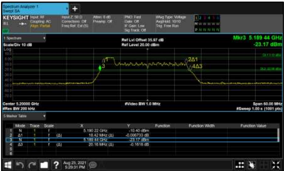
Figure 189 - Core 0 (A) 5200 MHz (CH40) 26 dB and 99% Bandwidth
