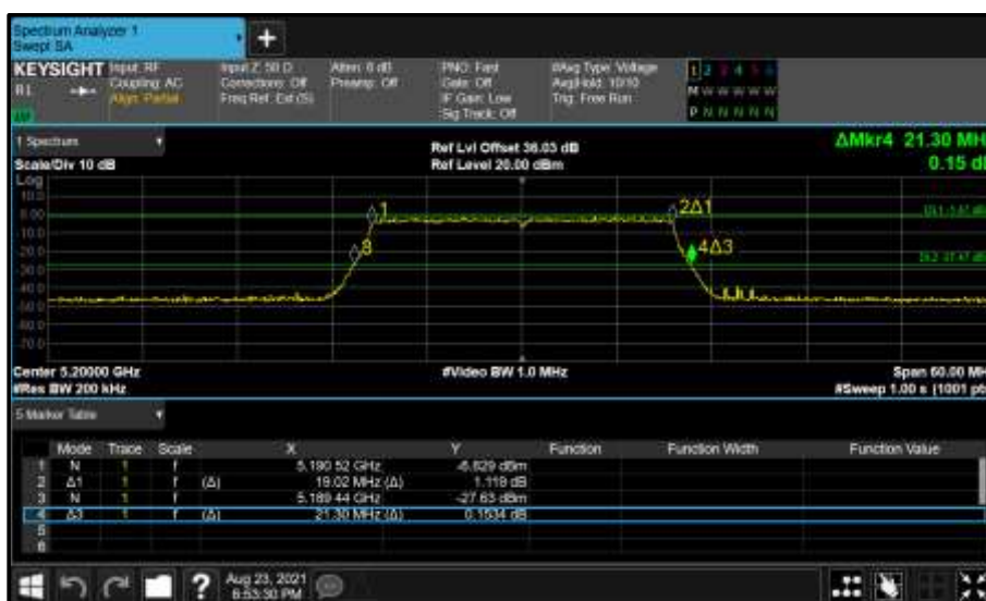
Figure 178 - Core 1 (B) 5200 MHz (CH40) 26 dB and 99% Bandwidth
