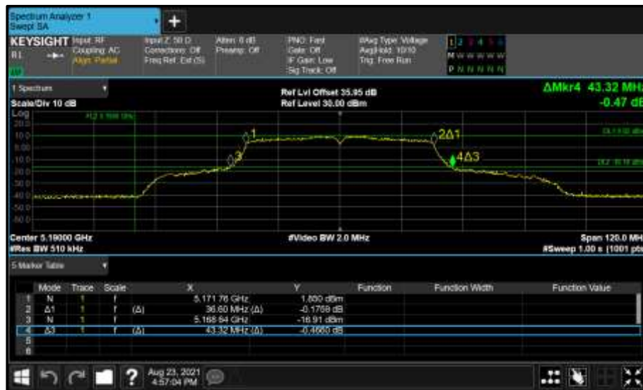
Figure 121 - Core 0 (A) 5190 MHz (CH38) 26 dB and 99% Bandwidth
