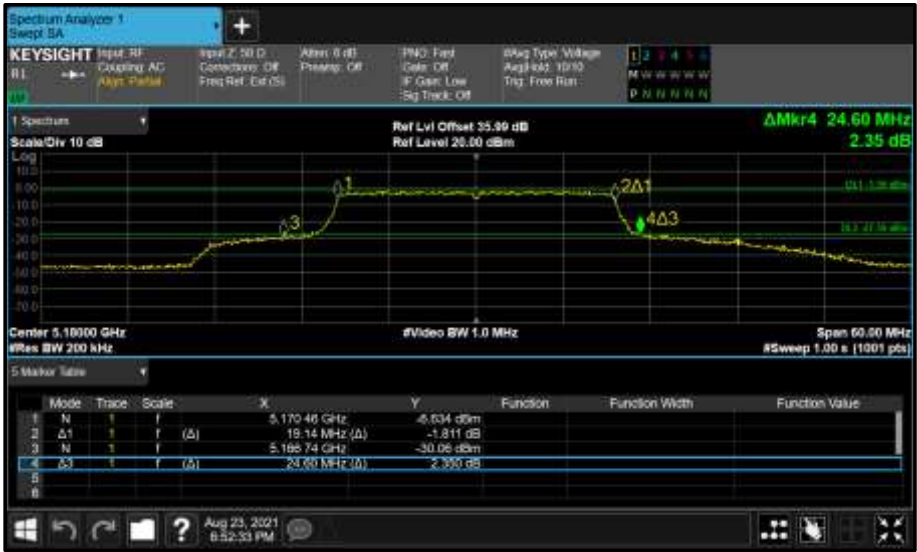
Figure 176 - Core 1 (B) 5180 MHz (CH36) 26 dB and 99% Bandwidth
