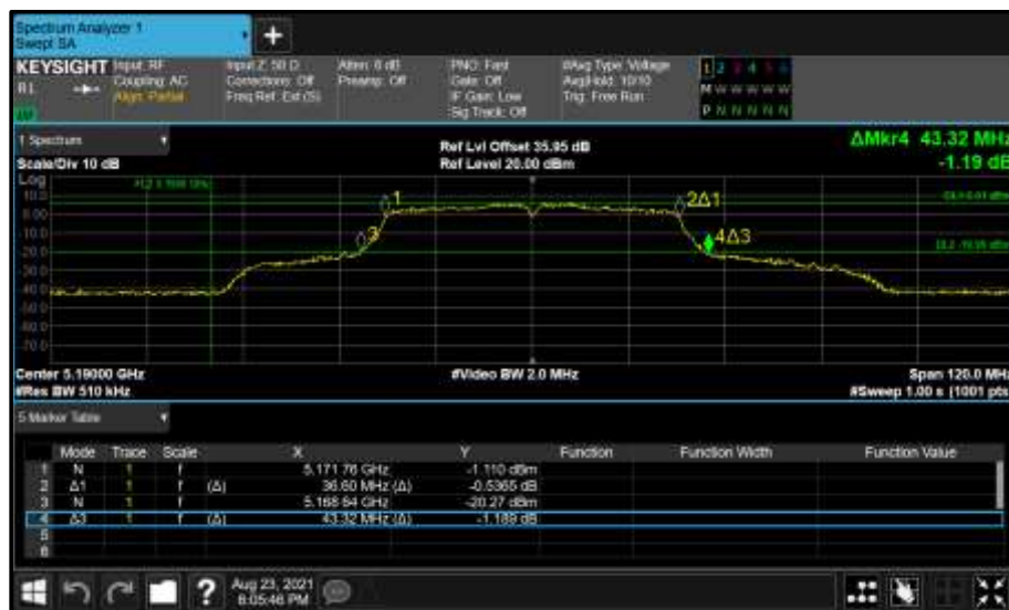
Figure 123 - Core 0 (A) 5190 MHz (CH38) 26 dB and 99% Bandwidth
