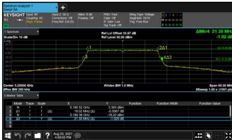
Figure 152 - Core 0 (A) 5200 MHz (CH40) 26 dB and 99% Bandwidth
