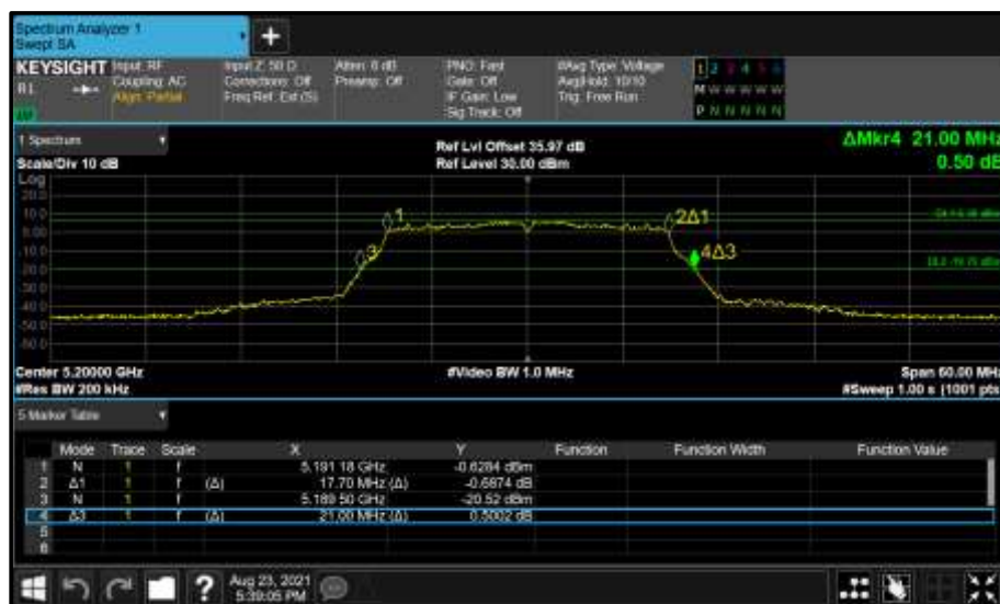
Figure 111 - Core 0 (A) 5200 MHz (CH40) 26 dB and 99% Bandwidth
