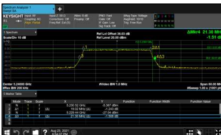
Figure 179 - Core 0 (A) 5240 MHz (CH48) 26 dB and 99% Bandwidth
