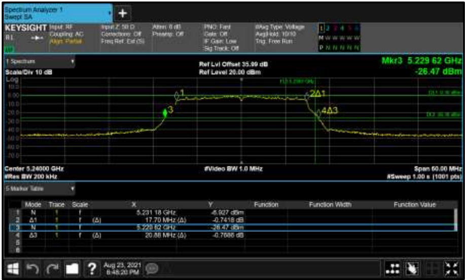
Figure 120 - Core 1 (B) 5240 MHz (CH48) 26 dB and 99% Bandwidth
