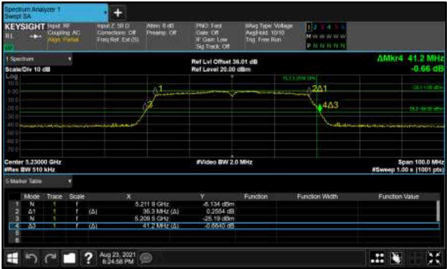
Figure 132 - Core 1 (B) 5230 MHz (CH46) 26 dB and 99% Bandwidth
