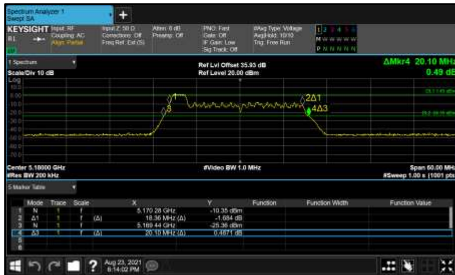
Figure 184 - Core 0 (A) 5180 MHz (CH36) 26 dB and 99% Bandwidth
