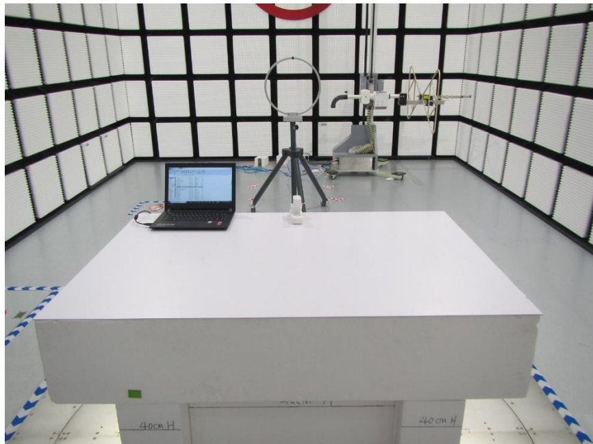
RADIATED RF MEASUREMENT SETUP (30MHz~1GHz)
