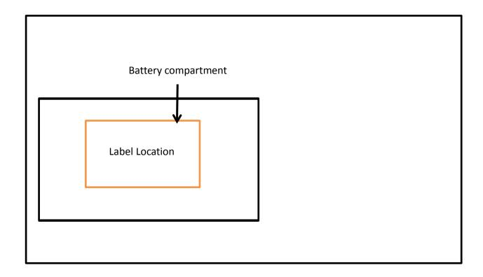
Label located in the battery compartment and is visible to the users as they install the battery.
