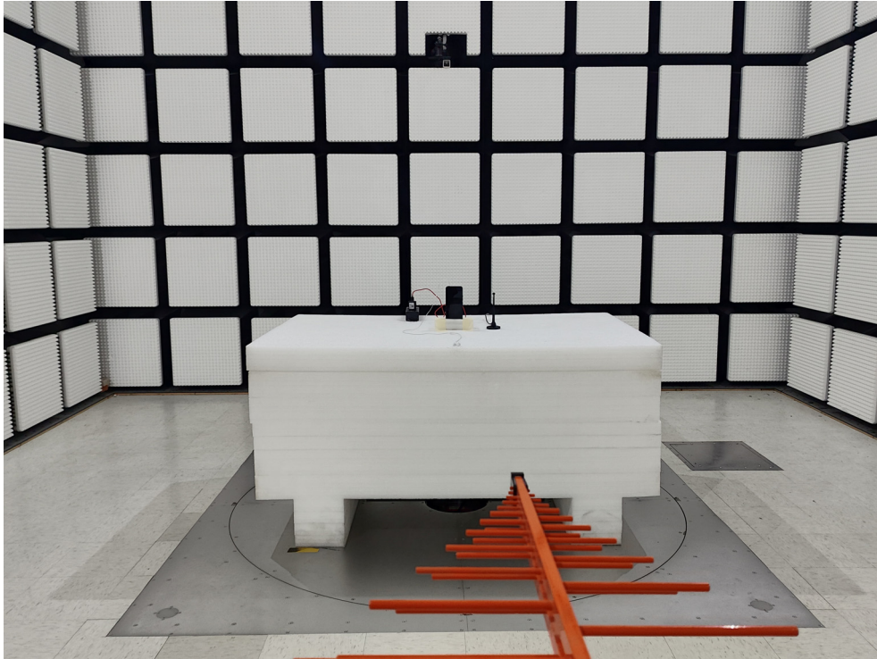
Radiated Emission Above 1GHz View-TX
