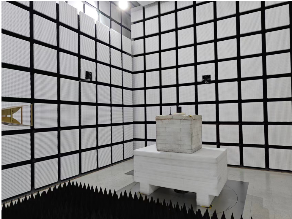
Radiated Emission Above 1GHz View-TX
