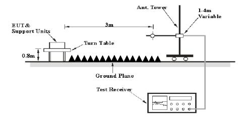
The radiated emission tests were performed in the 3 meters chamber test site A for the range 30MHz to 1GHz and the 3 meters chamber test site B for above 1GHz, using the setup accordance with the ANSI C63.4-2014. The specification used was the FCC Part 15.109 Class B limits.
