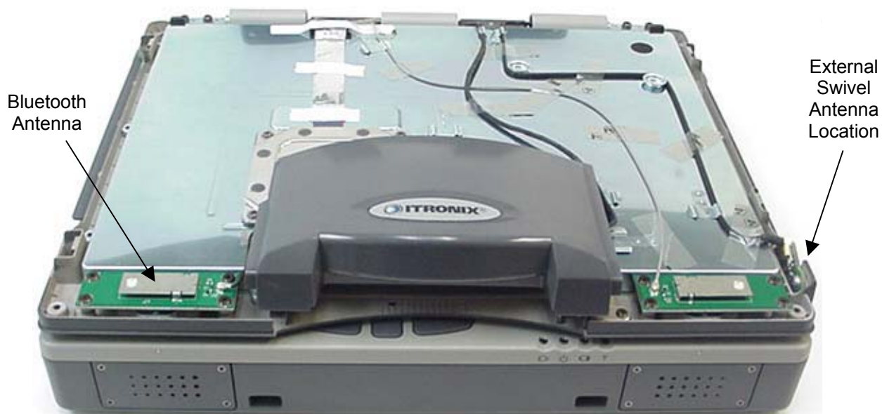
Photograph A-7 –Surface-Mount Antenna Placement
