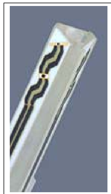
Inside view of ET3DV6 E-field Probe
