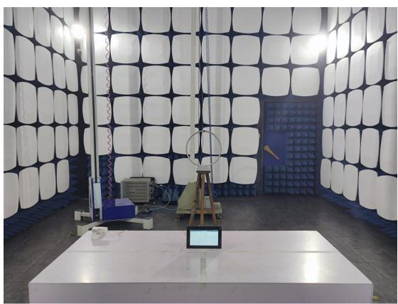
3. Radiated emission (9KHz-30MHz)
