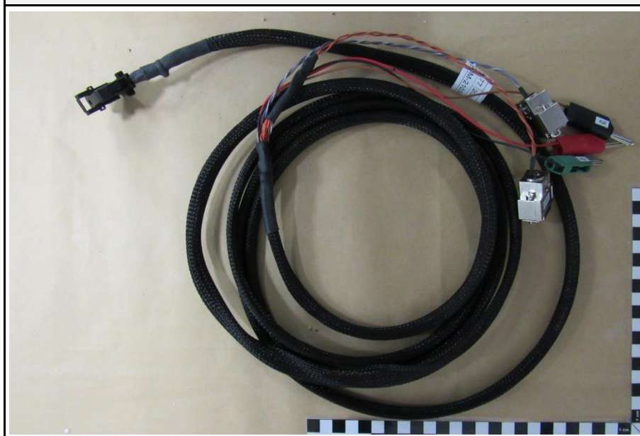
AE: Power and CAN cable
