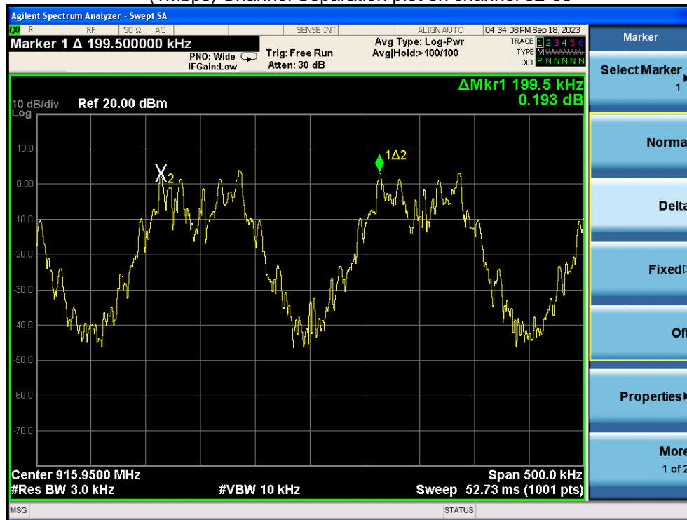
(1Mbps) Channel Separation plot on channel 102-103
