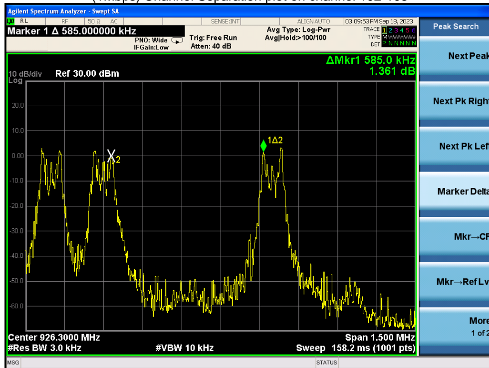
(1Mbps) Channel Separation plot on channel 102-103
