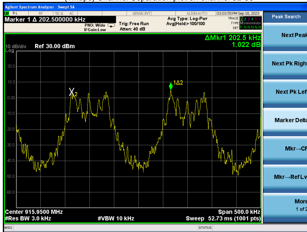
(1Mbps) Channel Separation plot on channel 102-103
