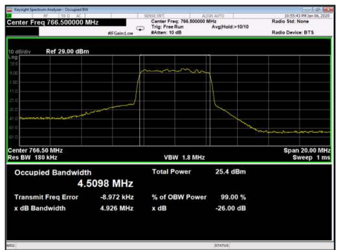
Figure 174: 64QAM 5MHz C.S; 766.5MHz, 15kHz Output
