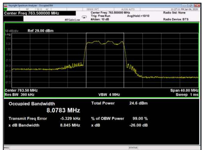
Figure 170: 16QAM 10MHz C.S; 763.5MHz, 60kHz Output
