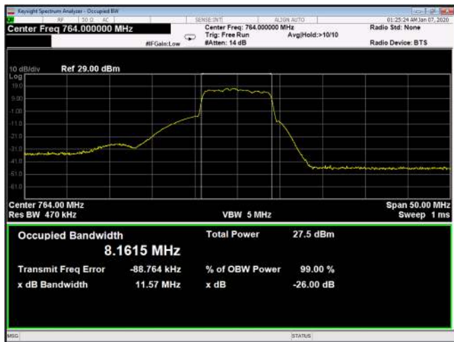
Figure 201: 256QAM 10MHz B.W.; 764.0MHz, 60kHz Output
