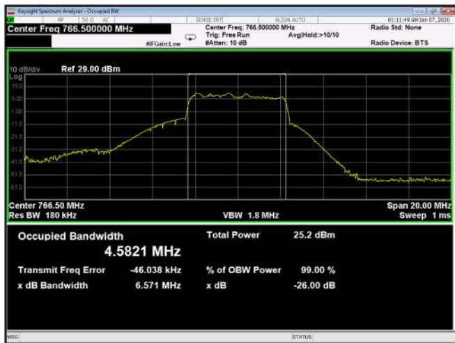
Figure 189: 256QAM 5MHz B.W.; 766.5MHz, 15kHz Output
