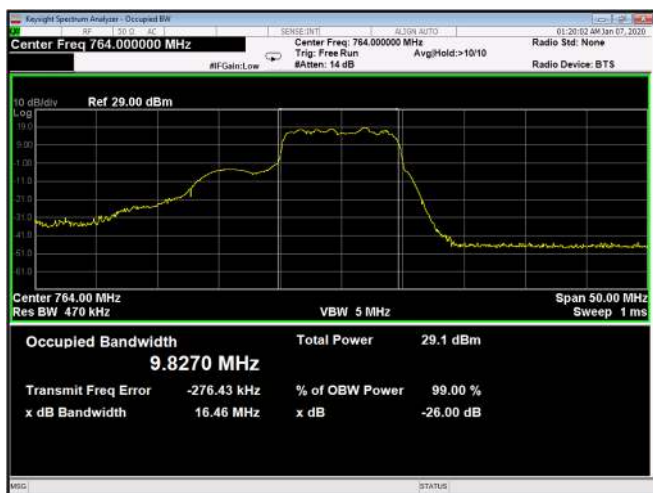
Figure 195: 256QAM 10MHz B.W.; 764.0MHz, 15kHz Output
