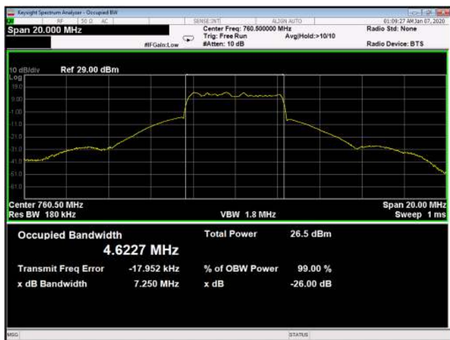
Figure 187: 256QAM 5MHz B.W.; 760.5MHz, 15kHz Output
