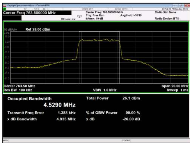
Figure 173: 64QAM 5MHz B.W.; 763.5MHz, 15kHz Output
