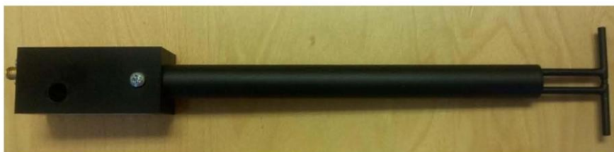
Figure 1 – MVG COMOSAR Validation Dipole
