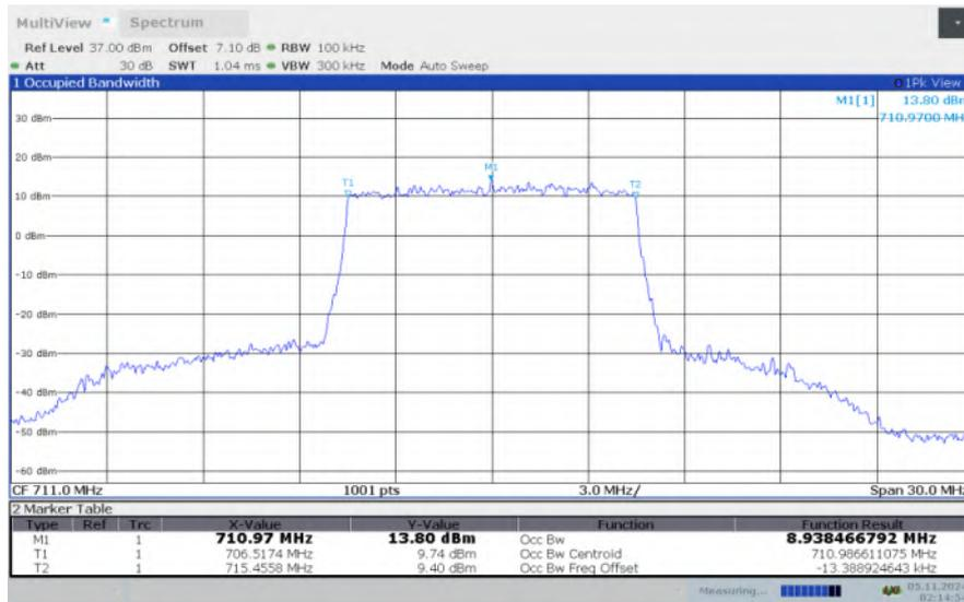
LTE band 17 , 10MHz Bandwidth, HIGH, 16QAM (99% BW)
