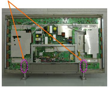
1. Apply a ferrite Core to the In/out Speaker cable and data cable
