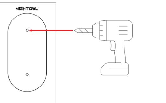
**NOTE:** A Power Drill, 15/64" (6mm) drill bit, mounting bracket, 15° mounting wedge (optional), and screw pack are required for mounting installation.
