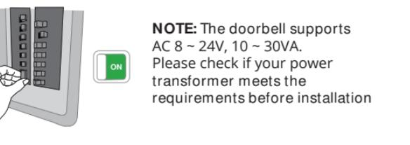
**NOTE:** The doorbell supports AC 8 ~ 24V, 10 ~ 30VA. Please check if your power transformer meets the requirements before installation
