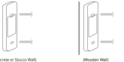
4. If installed on a wooden wall, no drilling is required, just use a screwdriver to install directly.
