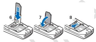
6 Direct the back cover towards the locking catches on the front cover (9), and slide the back cover until it locks into place (10).
