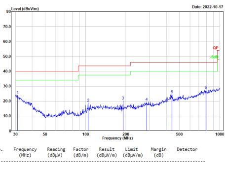
Test Mode: Transmitting Polarization: vertical Note:
