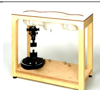
Fig 5.9 Photo of SAM Phantom
