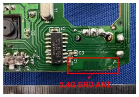
Antenna Length 12mm\*6mm Antenna Type: PCB Antenna Antenna Gain: 0dBi
