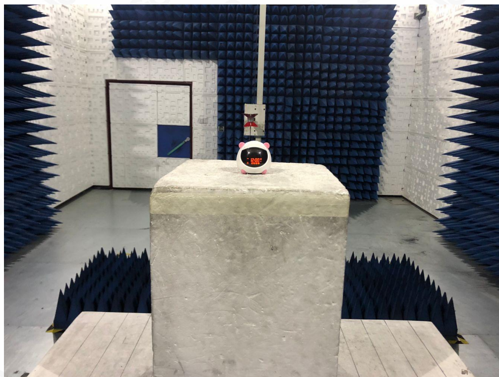
FCC RADIATED EMISSION TEST SETUP ABOVE 1GHZ
