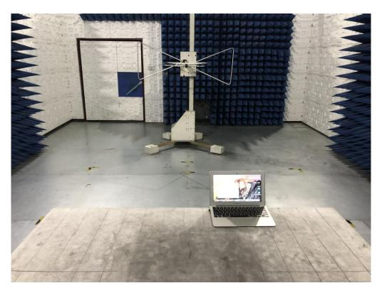
FCC RADIATED EMISSION TEST SETUP ABOVE 1GHZ
